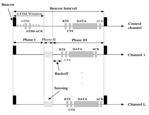
Fig. 4 Multichannel timing structure of OSA-MAC protocol for the distributed cognitive network [99]
