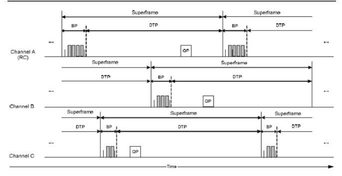
Fig. 3 The multichannel super-frame structures for C-MAC protocol in the distributed cognitive network as in [97]
