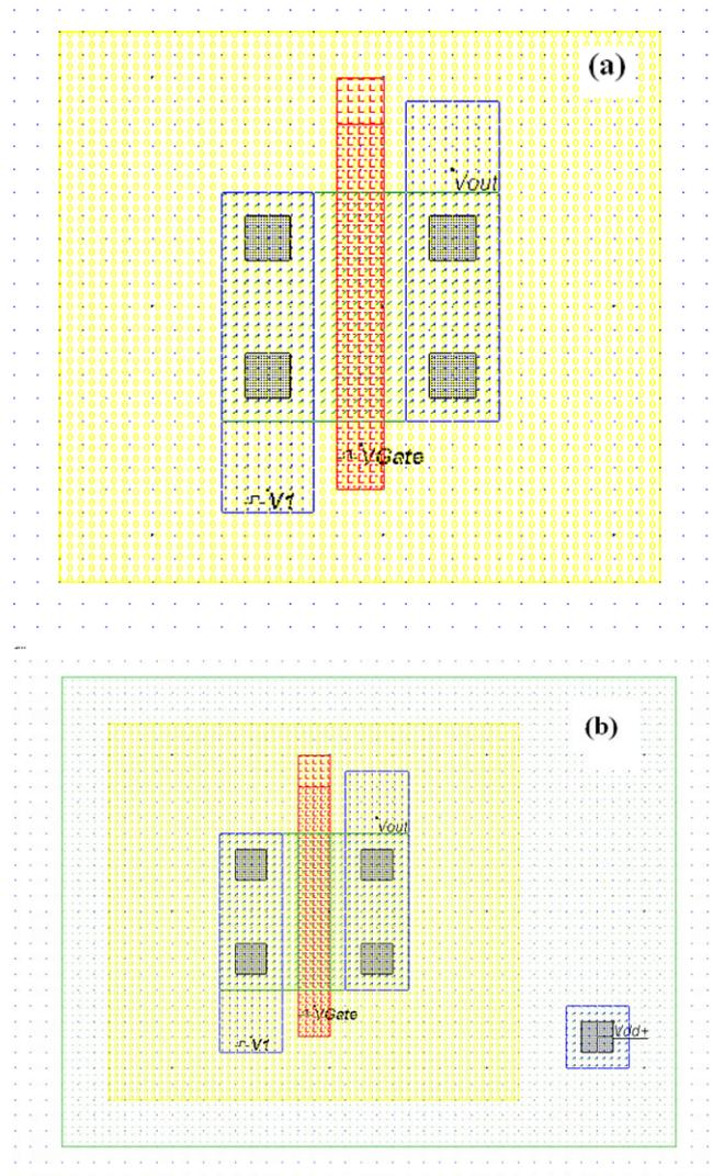
**Fig. 4** Layout of the (a) n-type DG MOSFET, and (b) p-type DG MOSFET
