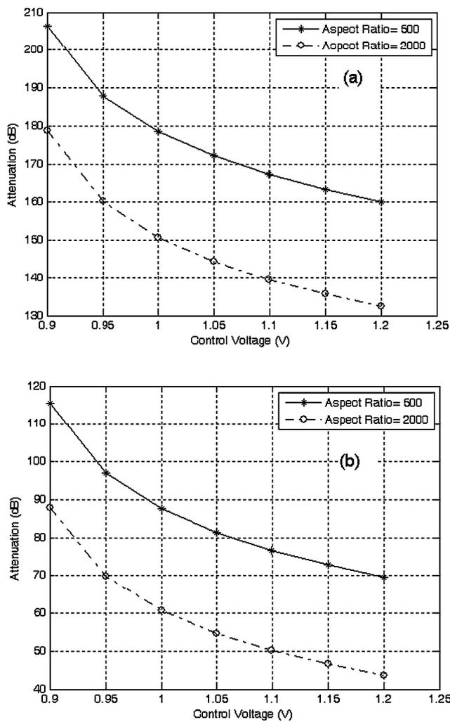
**Fig. 8** Attenuation at control voltage  $V_{CTL} = 1.2$  V for, (a) 0.8- $\mu$ m technology and (b) 45-nm technology
