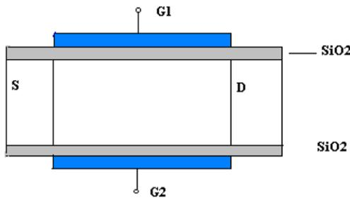
**Fig. 3** Schematic of the basic double-gate n-MOSFET
