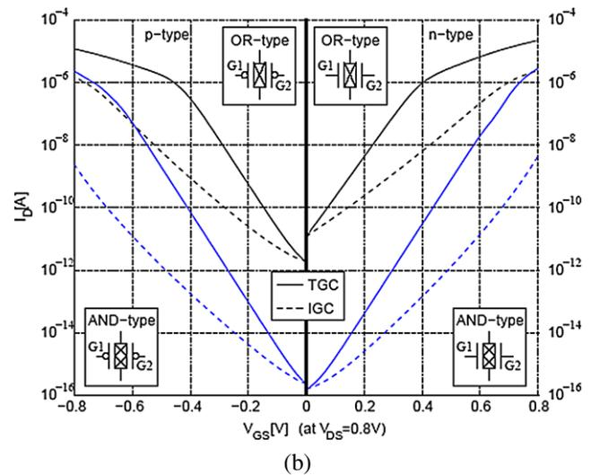
**Fig. 2** Conversion of the (a) series and parallel combination of n-MOSFET/p-MOSFET to DG MOSFET and (b) transfer characteristics of independent double-gate MOSFET [5]
