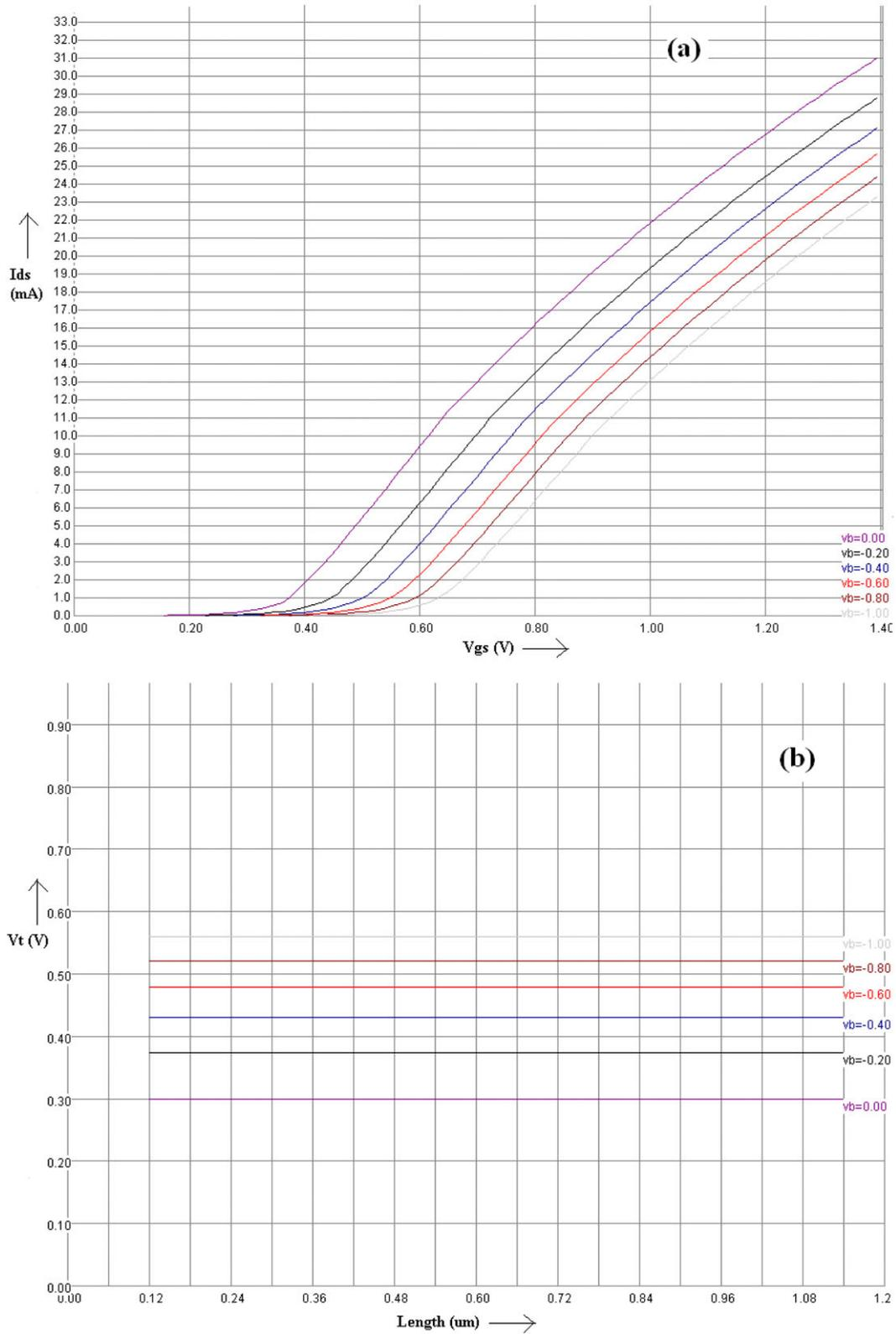
**Fig. 6** Characteristics of the (a) drain current with gate to source voltage, and (b) threshold voltage with the aspect ratio 500
