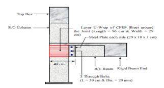
Fig. 12: B-C joint jacketing with mechanical anchorage system
