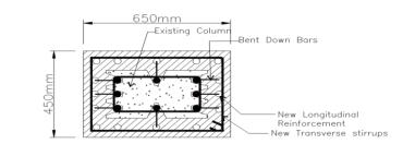
Fig. 8: Typical Section showing Column Jacketting
