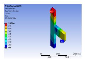
Fig. 10: Deformation after Jacketing
