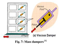
When seismic energy is transmitted through them, dampers absorb part of it, and thus damp the motion of the building. Some of the actual applications of these systems worldwide are given in Table 1. The most commonly used different types of dampers (Fig. 7) are:
