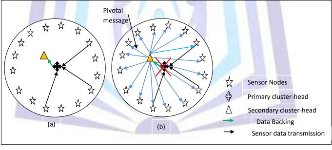
Figure 4 Working of Vital and Backup cluster-head
