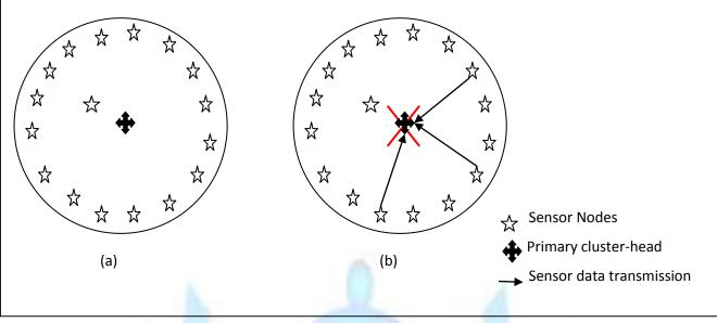
Figure 3 Non fault Tolerant sensor network
