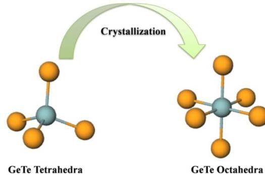
**Figure 1.14.** Alteration in *Ge* local structure from tetrahedral to octahedral on crystallization of amorphous *GST*.
