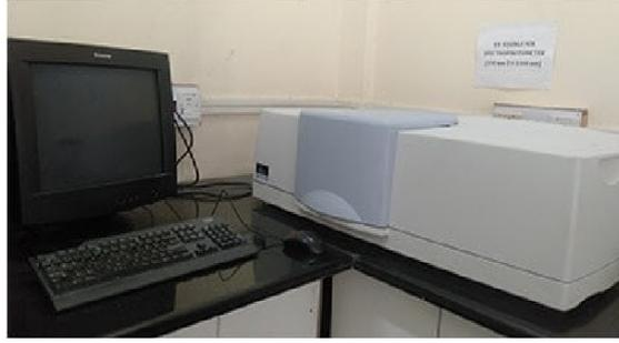
**Figure 3.12** *UV-Vis-NIR* spectrophotometer (model Perkin Elmer Lambda 750) used to measure optical transmission.
