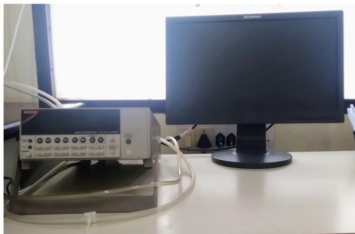
**Figure 3.14** Keithley 6487 electrometer used for the electrical measurements of prepared samples.
