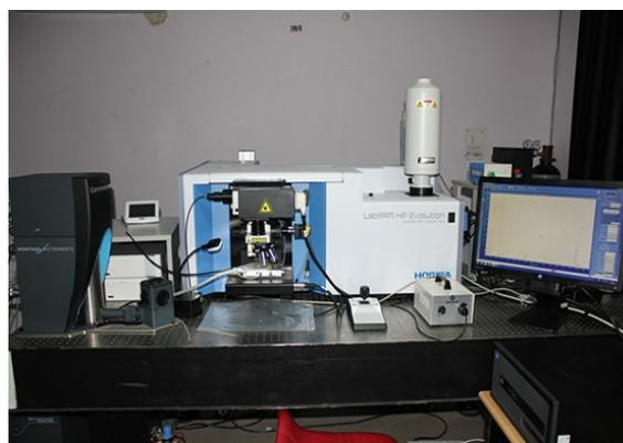
**Figure 3.10** Raman spectrometer model Horiba Jobin-Yvon LabRAM HR evolution (*IIT Mandi*) used for analysis.
