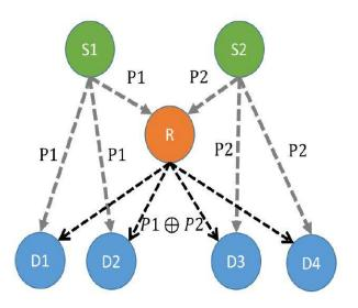
Figure 1: Network Coding using XOR
