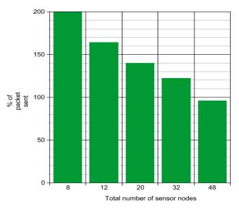
Figure 11: Total no. of packets sent with respect to no. of nodes
