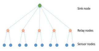
Figure 4: Network with Ten sensor nodes
