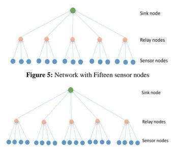
Figure 6: Network with Twenty sensor nodes
