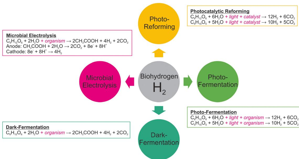
**Fig. 5** The possible chemical reactions to generate biohydrogen ( $H_2$ ) by conversion engineering of monosugars (glucose and xylose)
