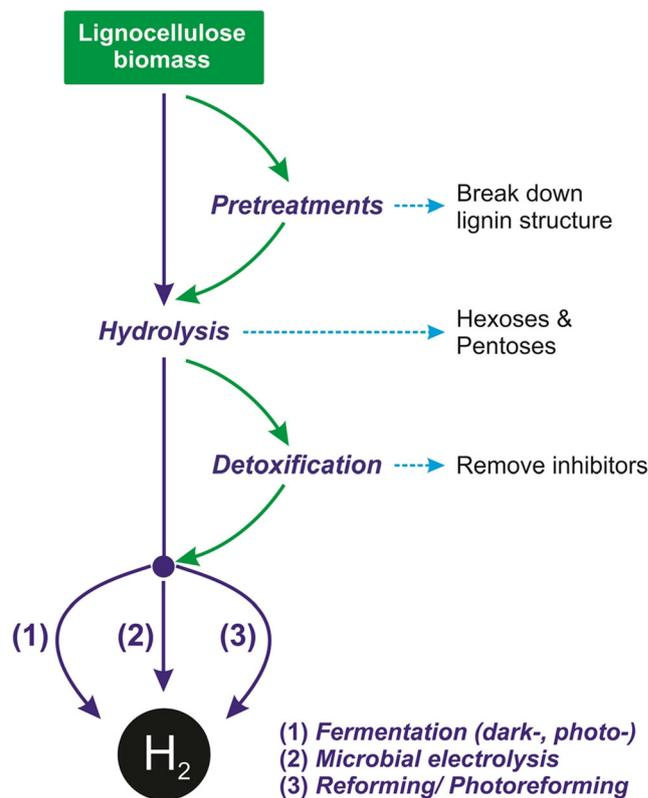
**Fig. 3** The outline of biohydrogen production from lignocellulosic-derived monosugars
