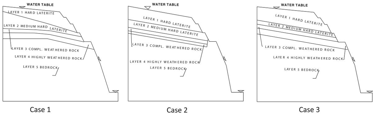
**Fig. 3** Different models of portal slope adopted for numerical study: Part I
