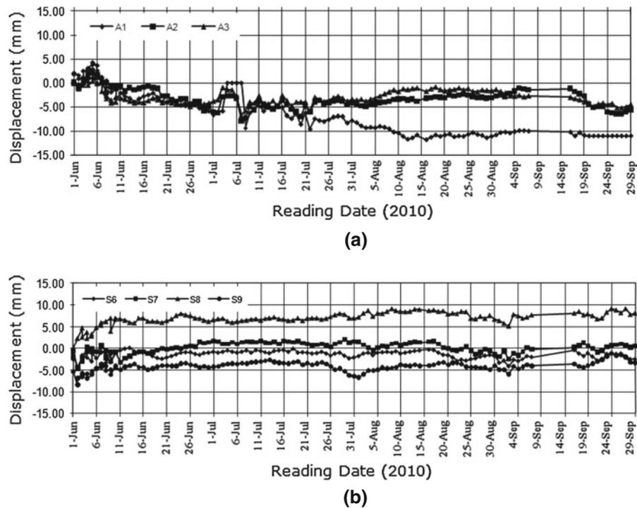
**Fig. 8** **a** Convergence monitoring above the centre of access tunnel. **b** Convergence monitoring on the right hand side of the access tunnel
