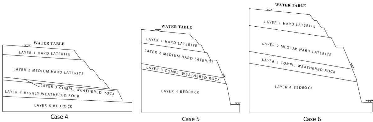
**Fig. 4** Different models of portal slope adopted for numerical study: Part II
