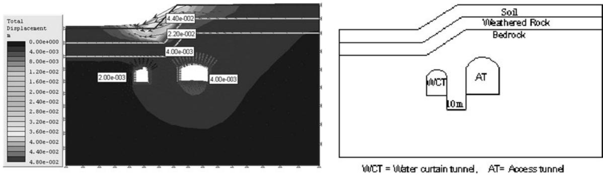
**Fig. 6** Model geometry along with total displacement contours after analysis (contours reported in metres)
