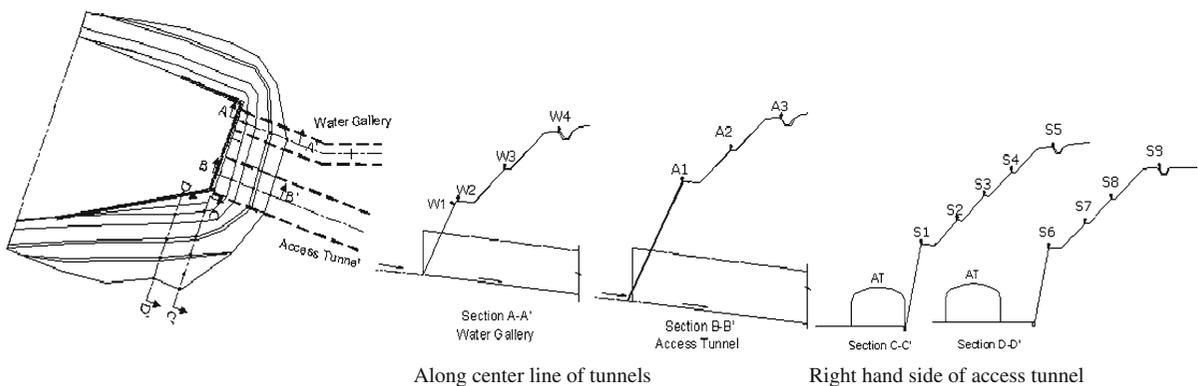
**Fig. 7** Optical survey target installation on slopes in portal area
