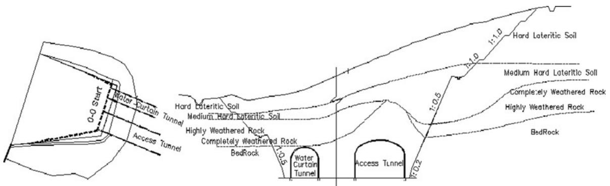
**Fig. 1** Plan and section of portal along with access tunnel and water curtain tunnel
