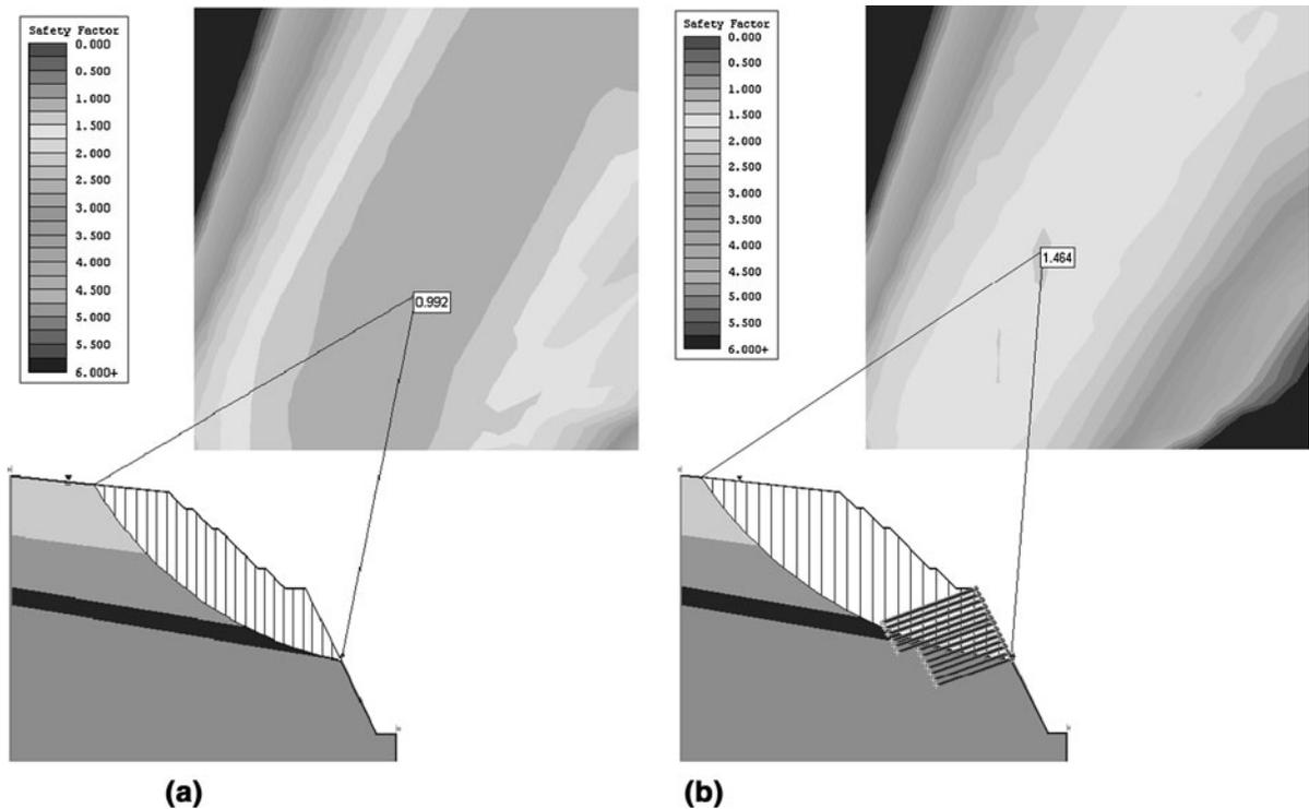
**Fig. 5** Critical slip surface obtained in limit equilibrium analysis **a** with and **b** without reinforcement for Case 6
