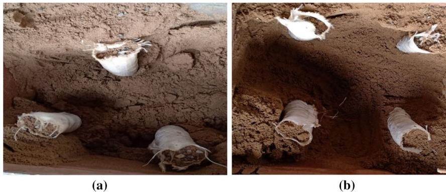
**Fig. 6** Exhumed vertically encased stone columns after group testing **a** 3 stone columns, **b** 4 stone columns
