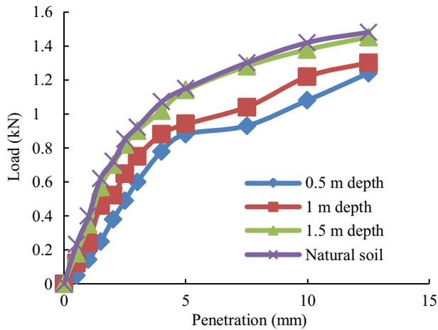
Fig. 26. Load vs. penetration curves (soaked) of dumpsite and natural soils from Solan.
