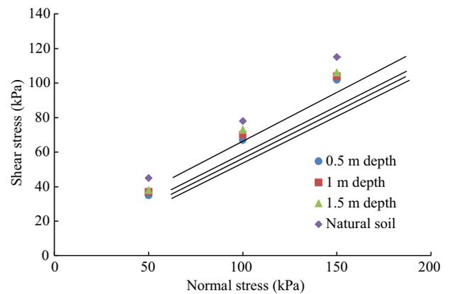
Fig. 6. Shear stress vs. normal stress curves of dumpsite and natural soils from Baddi.
