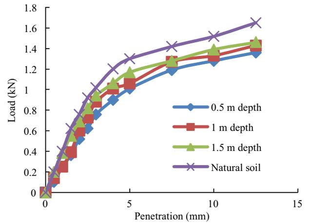
Fig. 5. Load vs. penetration curves (soaked) of dumpsite and natural soils from Baddi.
