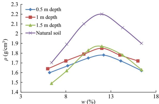
Fig. 28. Variations in maximum dry density with optimum moisture content of dumpsite and natural soils from Solan.
