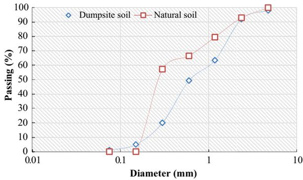
Fig. 2. Grain size analyses of dumpsite and natural soils from Baddi.
