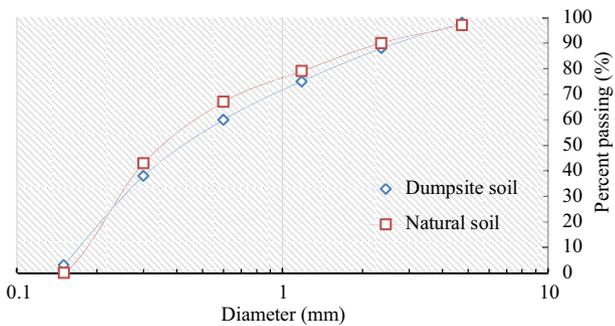
Fig. 16. Grain size analyses of dumpsite and natural soils from Sundernagar.
