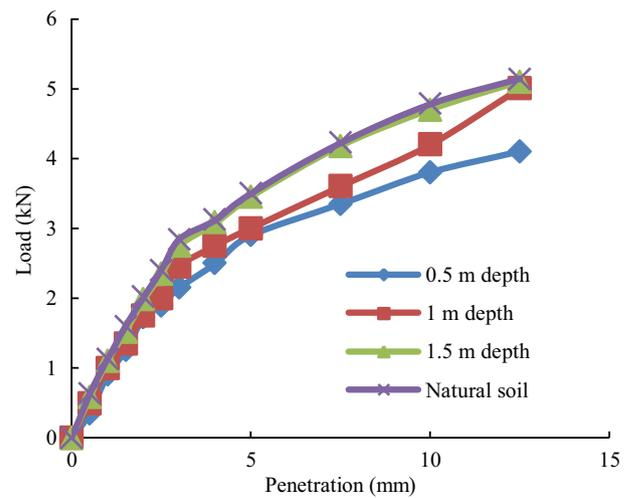
Fig. 18. Load vs. penetration curves (un-soaked) of dumpsite and natural soils from Sundernagar.
