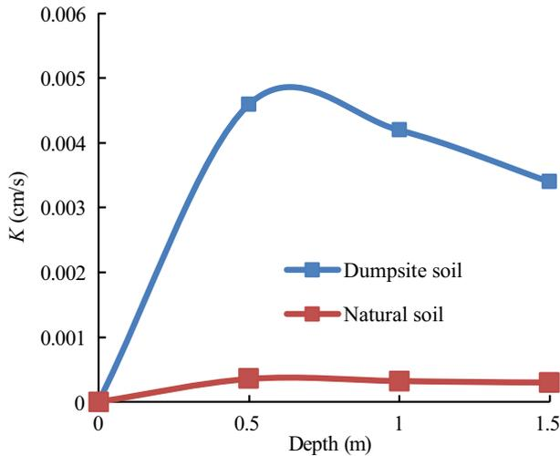
Fig. 22. Variations in hydraulic conductivity with depth of natural and dumpsite soils from Sundernagar.
