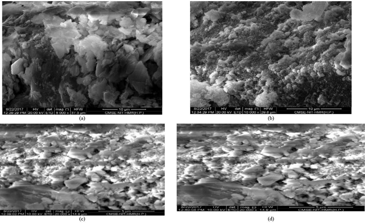
Fig. 30. SEM images of mineral particles in soil samples from Solan dumpsite.
