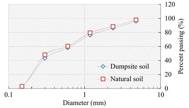
Fig. 23. Grain size analyses of dumpsite and natural soils from Solan.
