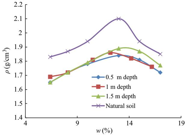
Fig. 14. Variations in maximum dry density with the optimum moisture content of dumpsite and natural soils from Mandi.
