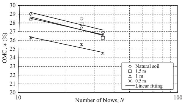
Fig. 10. Variations in optimum moisture content (OMC) with number of blows of dumpsite and natural soils from Mandi.
