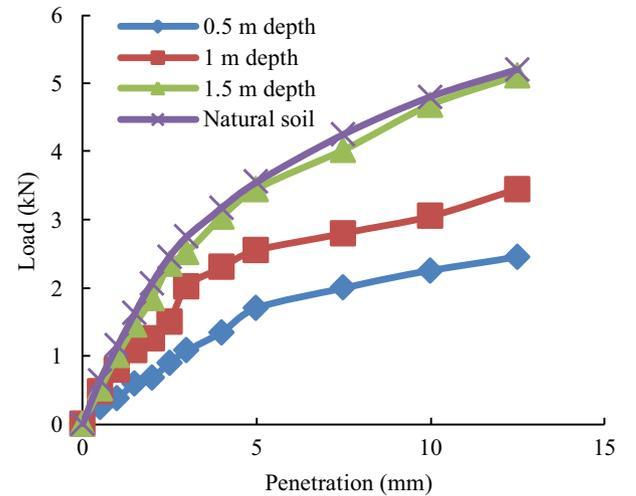
Fig. 25. Load vs. penetration curves (un-soaked) of dumpsite and natural soils from Solan.
