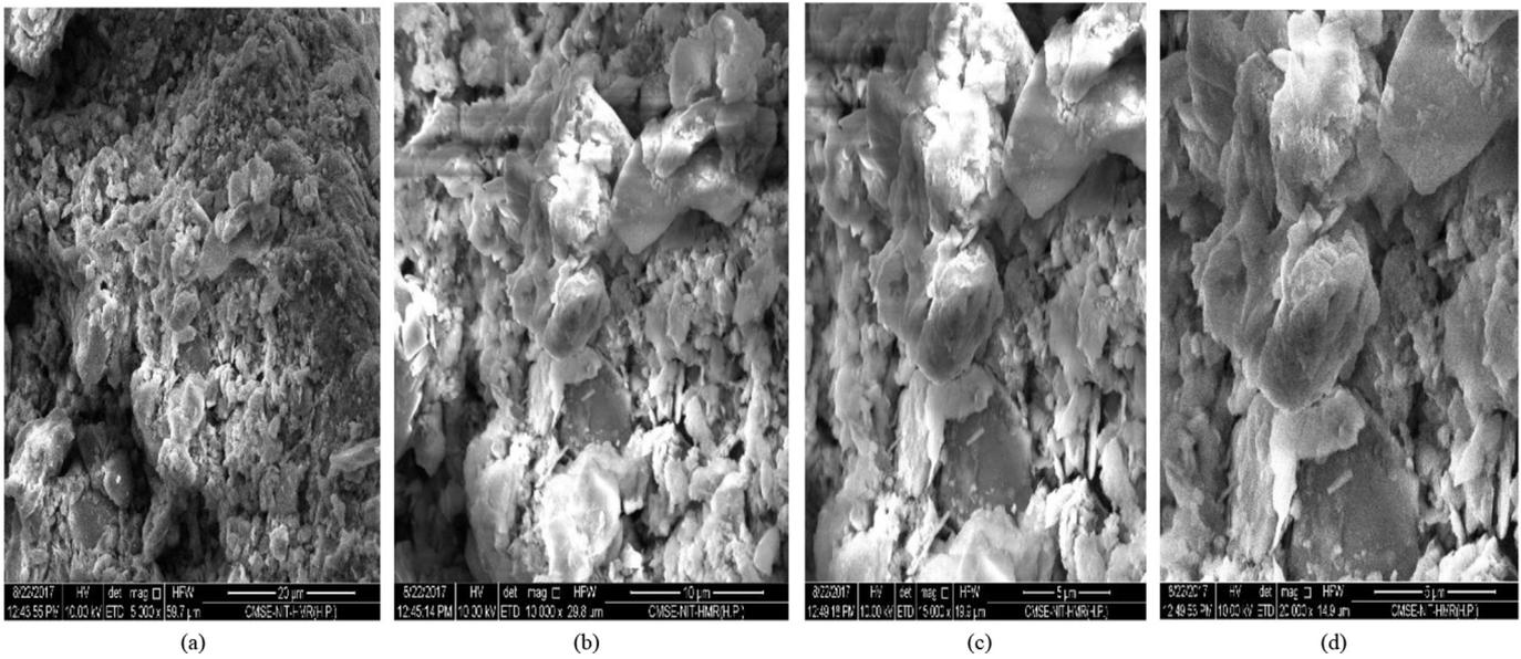
Fig. 32. SEM images of mineral particles in soil samples from Mandi dumpsite.
