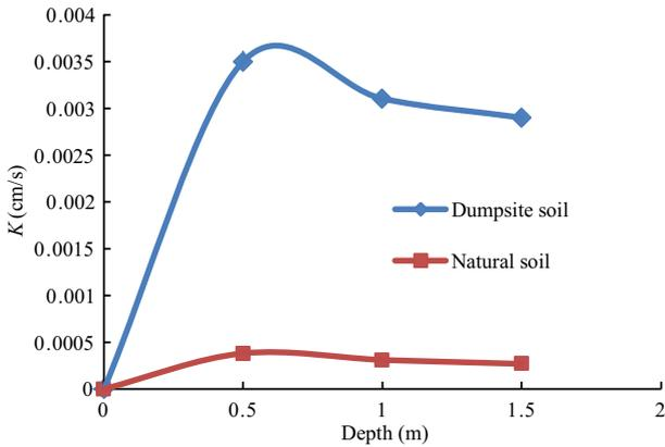
Fig. 8. Variations in permeability of natural and dumpsite soils from Baddi with depth.
