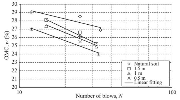
Fig. 17. Variations in optimum moisture content with number of blows of dumpsite and natural soils from Sundernagar.
