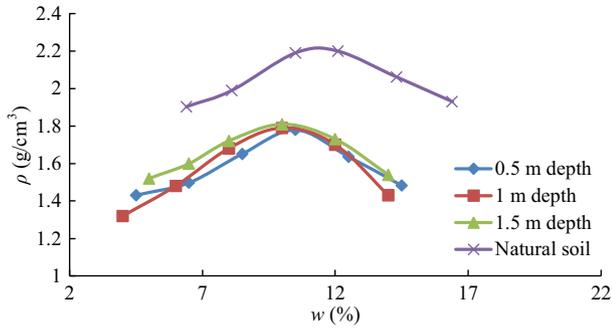
Fig. 7. Variations in maximum dry density with the optimum moisture content of dumpsite and natural soils from Baddi.
