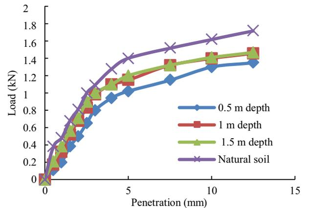
Fig. 19. Load vs. penetration curves (soaked) of dumpsite and natural soils from Sundernagar.
