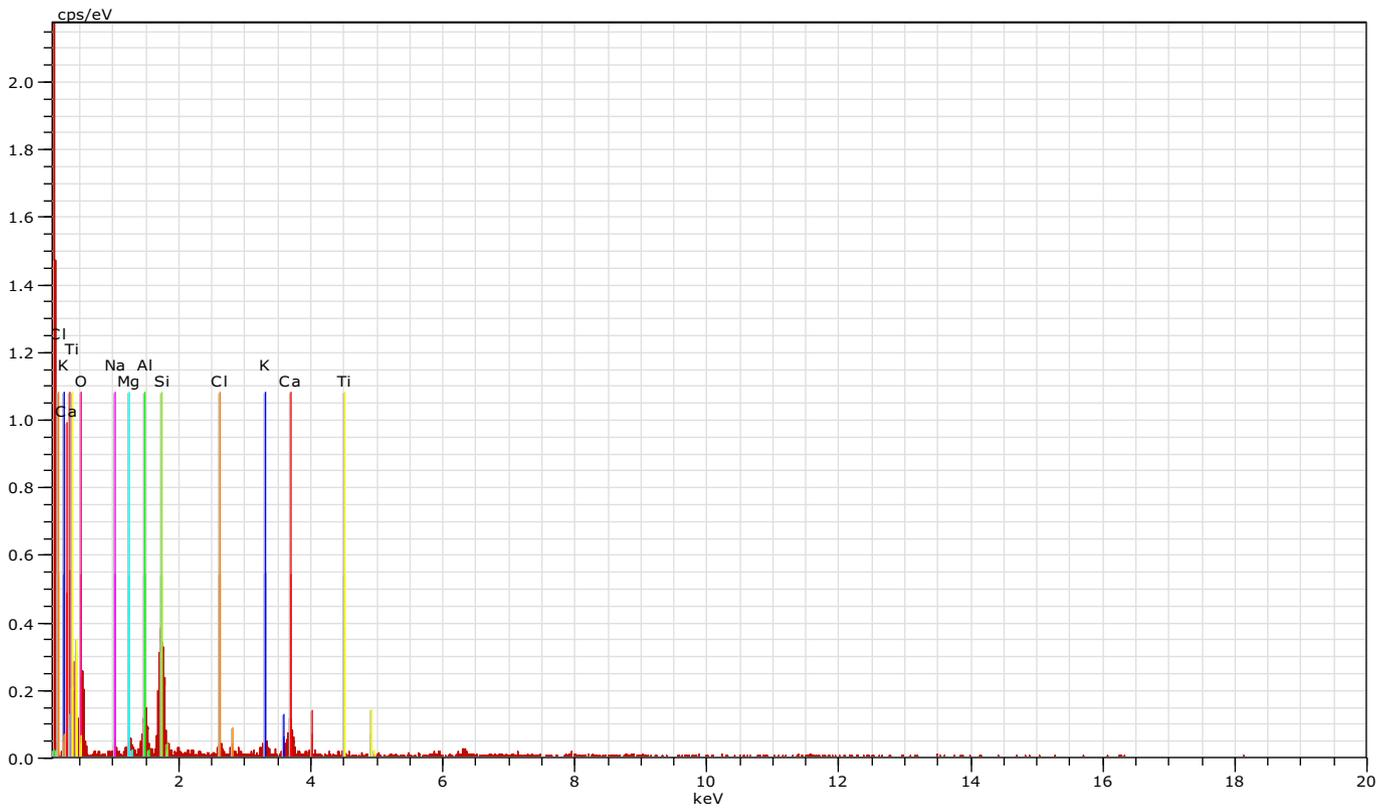
Fig. 31. EDS analysis data of soil samples from Solan dumpsite.
