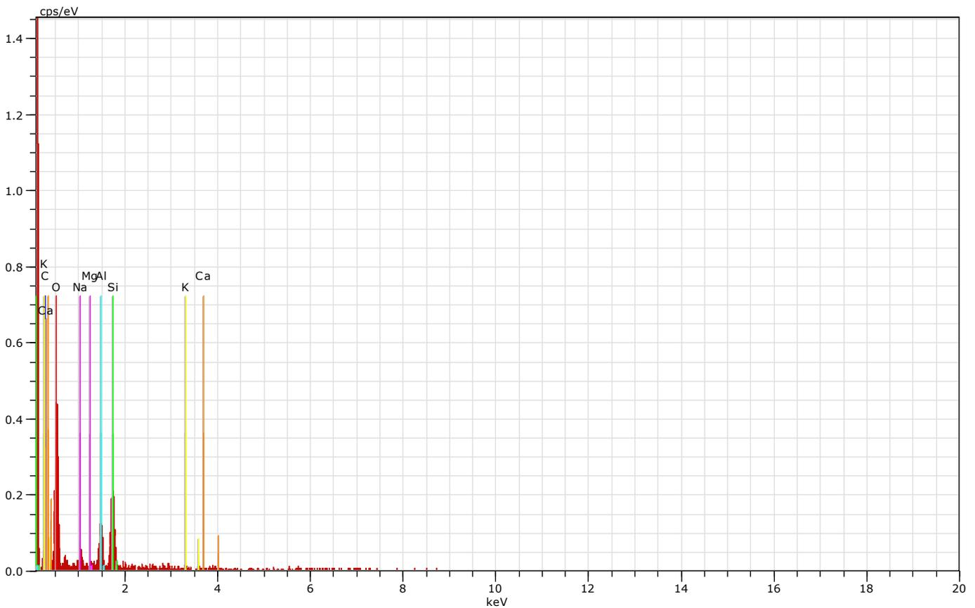
Fig. 37. EDS analysis data of soil samples from Baddi dumpsite.
