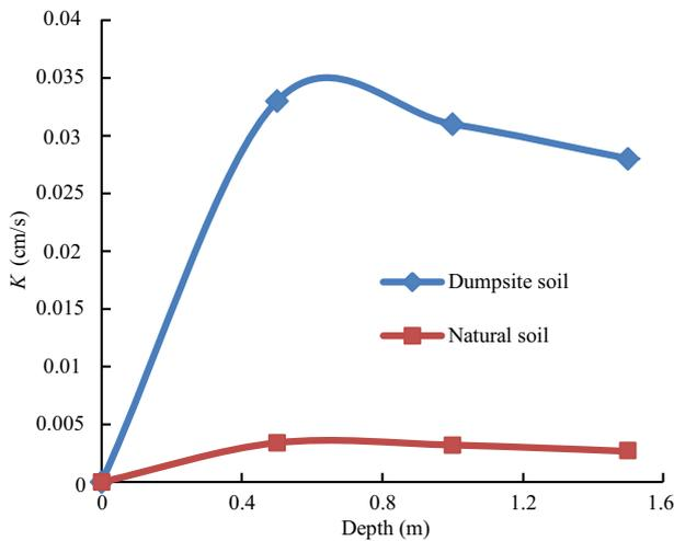
Fig. 15. Variations in hydraulic conductivity with depth of natural and dumpsite soils from Mandi.
