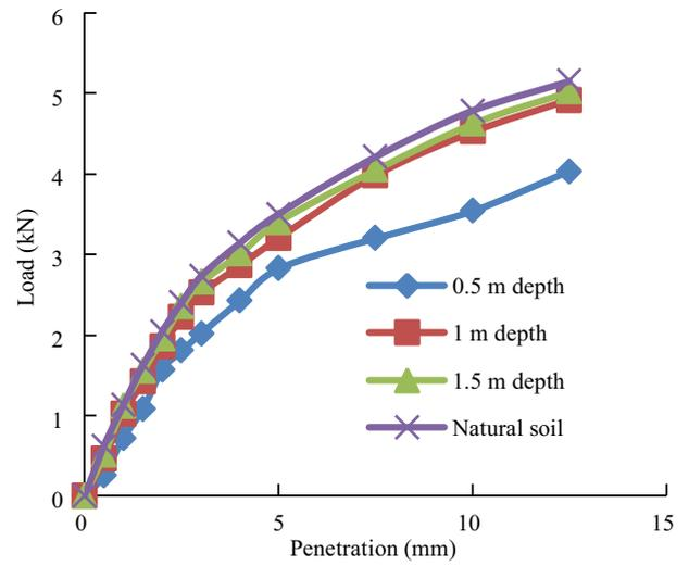
Fig. 4. Load vs. penetration curves (un-soaked) of dumpsite and natural soils from Baddi.
