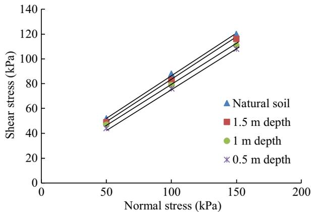
Fig. 27. Shear stress vs. normal stress curves of dumpsite and natural soils from Solan.
