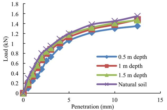
Fig. 12. Load vs. penetration curves (soaked) of dumpsite and natural soils from Mandi.
