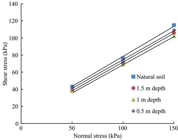
Fig. 20. Shear stress vs. normal stress curves of dumpsite and natural soils from Sundernagar.
