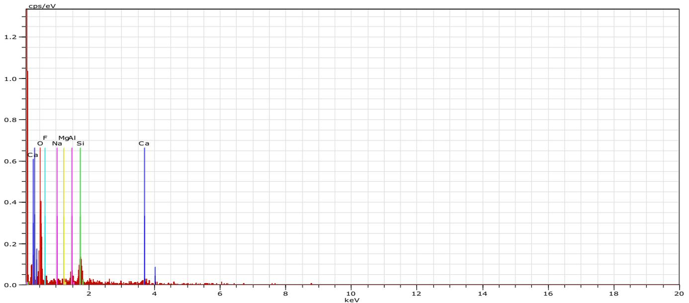
Fig. 35. EDS analysis data of soil samples from Sundernagar dumpsite.
