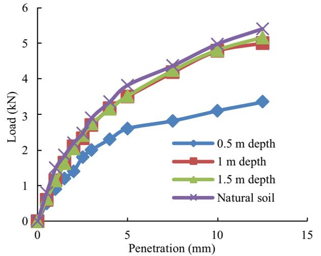
Fig. 11. Load vs. penetration curves (un-soaked) of dumpsite and natural soils from Mandi.
