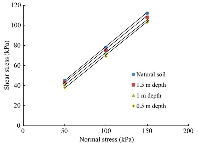
Fig. 13. Shear stress vs. normal stress curves of dumpsite and natural soils from Mandi.
