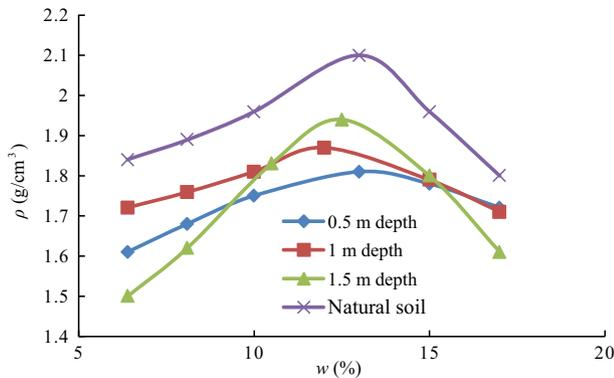
Fig. 21. Variations in maximum dry density with the optimum moisture content of dumpsite and natural soils from Sundernagar.
