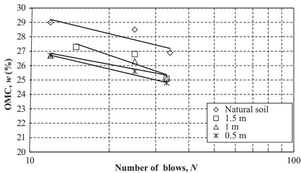
Fig. 3. Variations in optimum moisture content (OMC) with number of blows of dumpsite and natural soils from Baddi.
