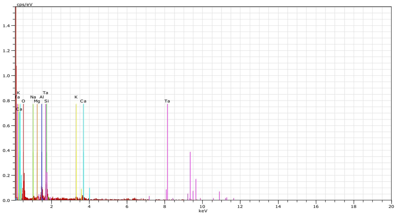
Fig. 33. EDS analysis data of soil samples from Mandi dumpsite.
