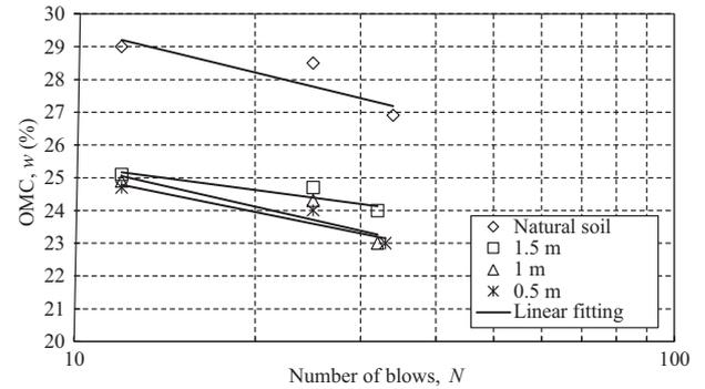
Fig. 24. Variations in optimum moisture content with number of blows of dumpsite and natural soils from Solan.
