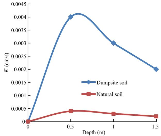
Fig. 29. Comparison in variation of hydraulic conductivity with depth of natural and dumpsite soils.
