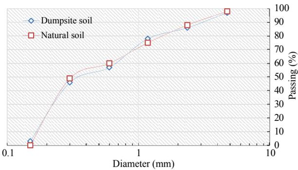
Fig. 9. Grain size analyses of dumpsite and natural soils from Mandi.
