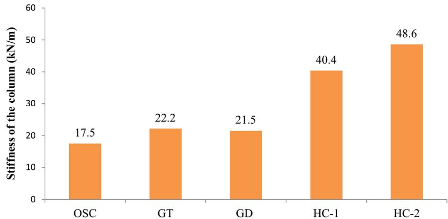
**Fig. 10** Variation of stiffness improvement factor with stone column encasement
