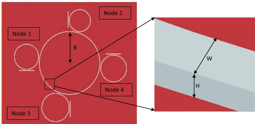
Fig. 4 SiO<sub>2</sub> waveguide network between Node 1, Node 2, Node 3 and Node 4 over Si substrate
