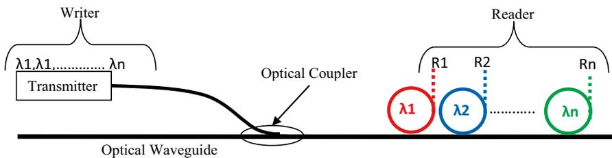
Fig. 5 SWMR physical organization optical resources needed for transmitter and receiver
