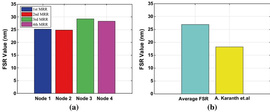
Fig. 7 FSR of micro-ring resonator. **a** FSR of four micro-ring resonators used in the proposed architecture. **b** Comparison between avg. FSR of four micro-rings compared to [22]
