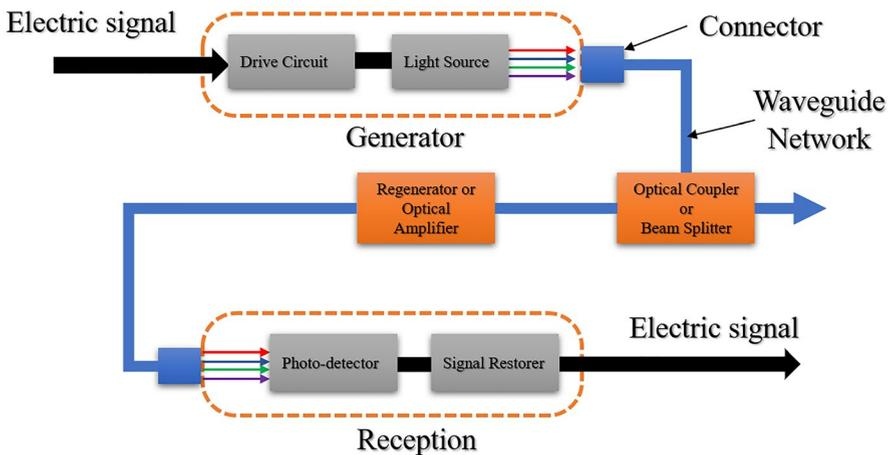
**Fig. 1** A photonic integrated circuit communication system
