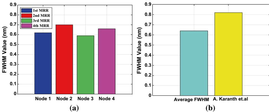
Fig. 8 FWHM of micro-ring resonator. **a** FWHM of four micro-ring resonators used in the proposed architecture. **b** Comparison between avg. FWHM of four micro-rings compared to [22]
