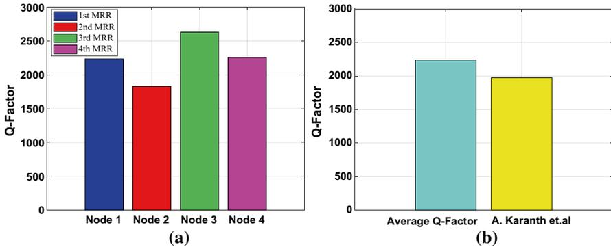
**Fig. 9** *Q*-factor of micro-ring resonator. **a** *Q*-factor of four micro-ring resonators used in the proposed architecture. **b** Comparison between avg. *Q*-factor of four micro-rings compared to [22]
