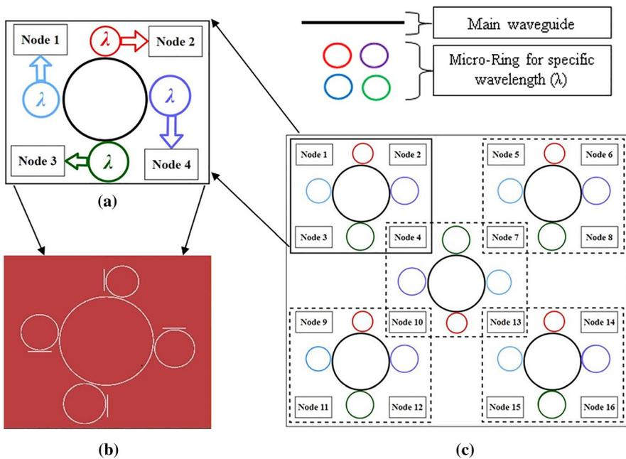
**Fig. 2** a Graphical representation of one cluster of nodes as brick, b simulated proposed architecture and c 4x4 2D architectural design for NoC
