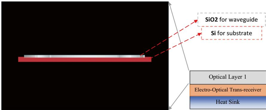
Fig. 3 Side view of architecture consists of SiO<sub>2</sub> as waveguide and Si for substrate
