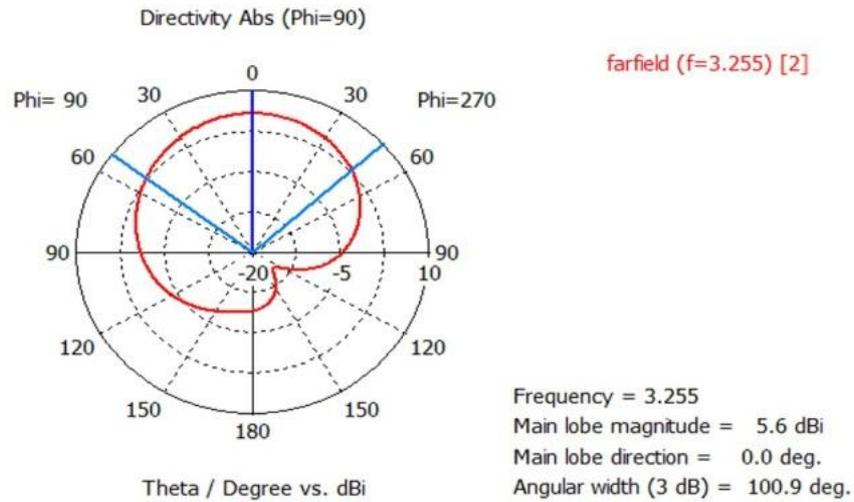
Figure 7: Far field for antenna 2
