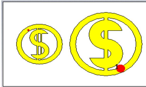
Figure 1: Top view of Basic configuration of patch antenna
