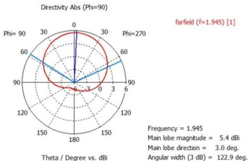
Figure 6: Far field for antenna 1
