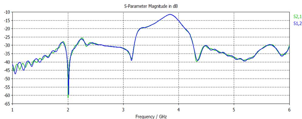
Figure 4: S12 and S21 parameters for two antennas.
