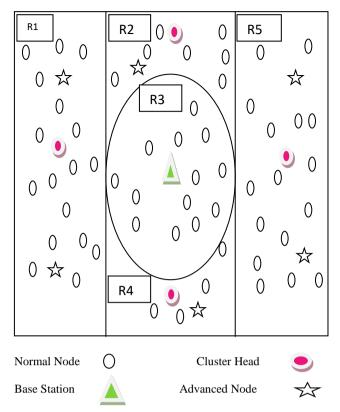
Figure 2: Heterogeneous Wireless Sensor Networks Architecture
