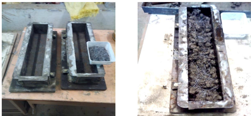
Fig. 3. Concrete beams with varying % of steel fibers.
