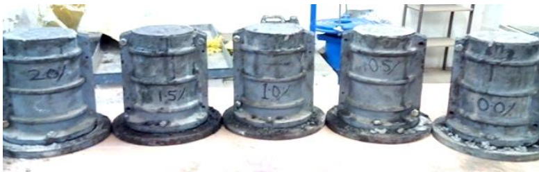
Fig. 2. Concrete cylinders with varying % of steel fibers.
