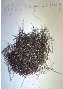
(c) 1.5% steel fibers of total volume fraction of concrete
