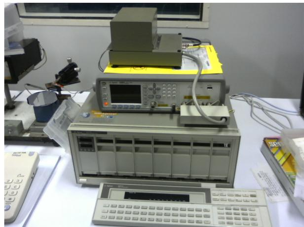
**Figure 1. Agilent E4980A LCR meter.**
