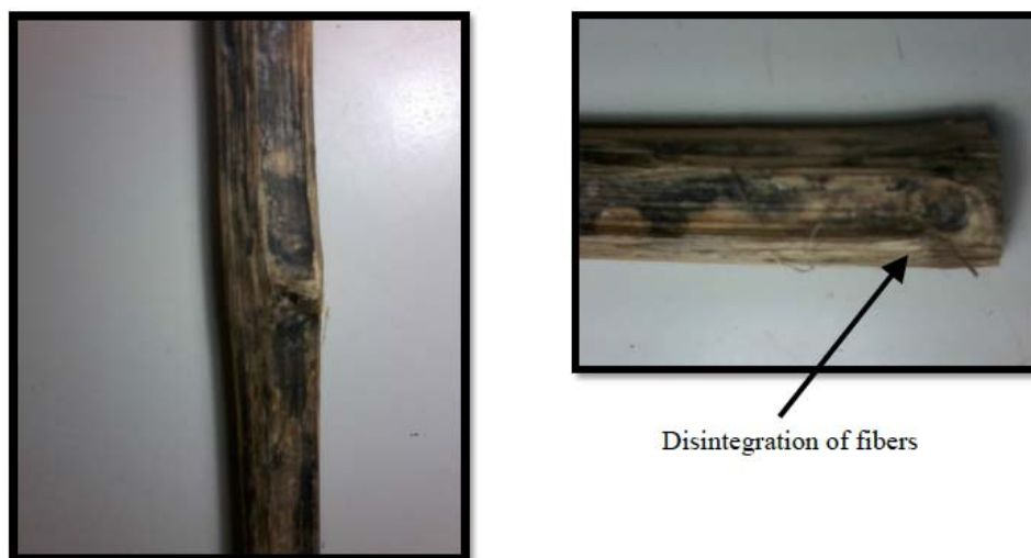
Figure 9: showing heavy fungal attack on the surface of one of the bamboo splint (W-1), soaked in water, causing rotting of bamboo & disintegration of fibers
