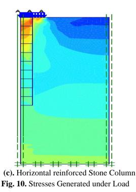
When three cases are compared, stress generated shows that most prominent case of unreinforced stone column is shown by red portion whereas least distinguished portion is shown by vertical reinforced stone column. This signifies that stresses which are generated in case of un-reinforced stone columns is comparatively more than that of reinforced stone column.
