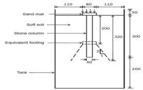
Fig. 3. Isolated stone column Schematic view
