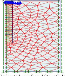
(c). Horizontally reinforced Stone Columns Fig. 8. Deformation under loads
