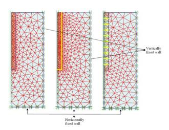
Fig. 7. Generated Initial Mesh
