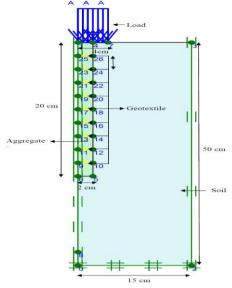
(c.) Geometry of model having structural elements in all.Fig. 6.
