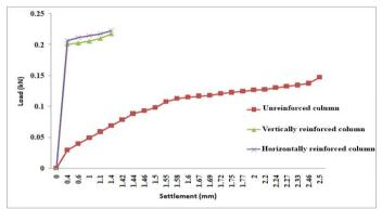
Fig. 9. Behaviour of Load versus settlement from
