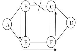
**Fig. 1.** An example of proposed link based recovery scheme (PLBRS).
