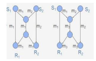
Figure 2: Butterfly Network; Source S<sub>1</sub> and S<sub>2</sub> multicast m<sub>1</sub> and m<sub>2</sub> to both receivers
