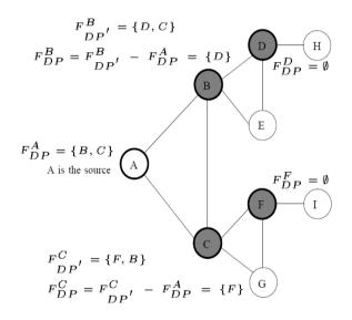
Figure 5: Failure of dominant pruning algorithm
