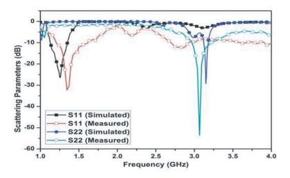
Figure 2. Scattering parameters of the antenna.
