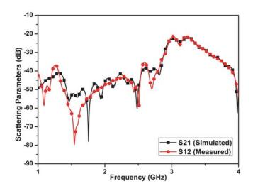
Figure 3. Isolation between patch antennas.
