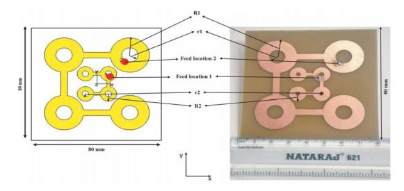
Figure 1. Layout of simulated and fabricated antenna.
