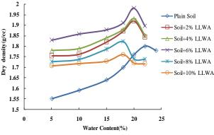
Fig. 3. Variation of dry density with moisture content for different LLWA contents
