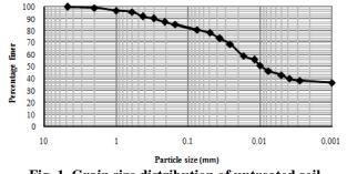
Fig. 1. Grain size distribution of untreated soil
