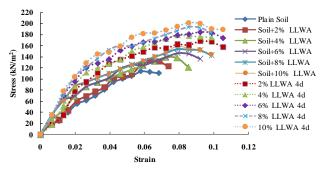
Fig. 4. Stress vs strain relation for uncured and 4 day cured soil mix
