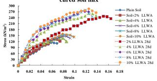
Fig. 5. Stress vs strain relation for uncured and 28 day cured soil mix
