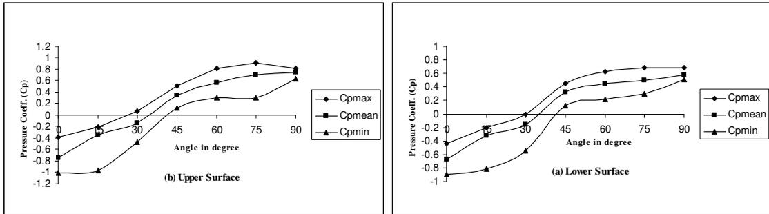
Figure 3 Plots of pressure coefficients on canopy of model HC-150
