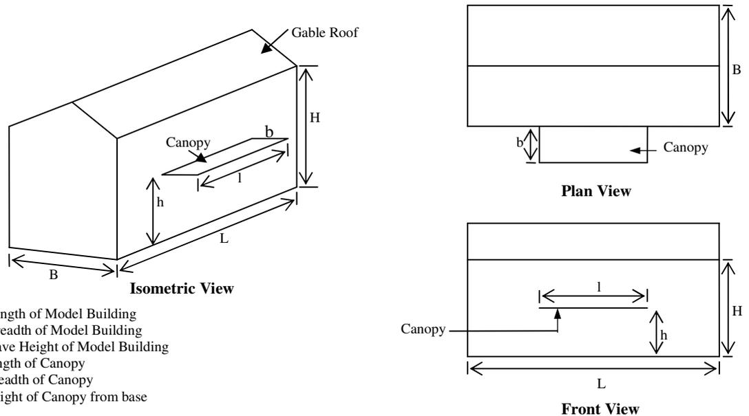
Figure 1 Model detail of gable roof building with attached canopy
