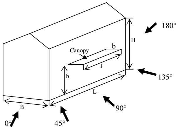
Figure 2 Angle of attack of wind on model
