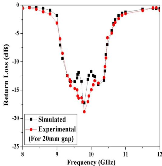
Fig. 3. Return-loss (in dB) variation with frequency (in GHz) for the sectoral patch at a gap of 20 mm.
