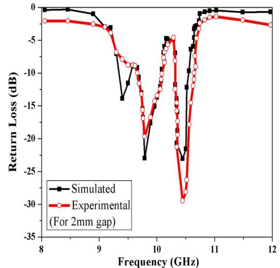
Fig. 2. Return-loss (in dB) variation with frequency (in GHz) when the four sectoral patches are unmoved (with 2-mm gap).
