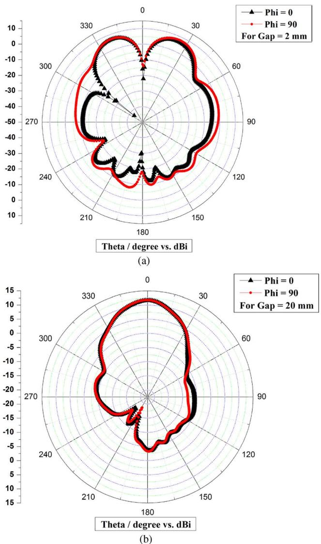
Fig. 4. Radiation pattern Directivity Abs ( $\Phi = 0$  and  $90$ ) between Theta degree versus dBi. (a) For gap = 2 mm. (b) For gap = 20 mm.
