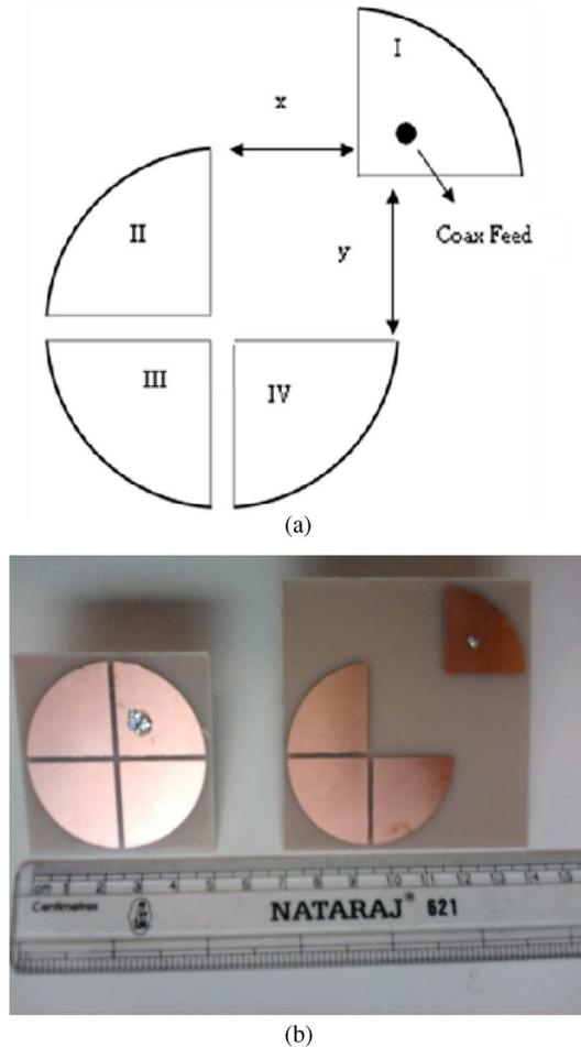
Fig. 1. Antenna design of sectoral patch antenna. (a) Geometry. (b) Prototype.
