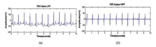
Fig. 4. Filtered ECG signal using FIR Kaiser Window(a) LPF for PLI removal (b) HPF for BLW removal
