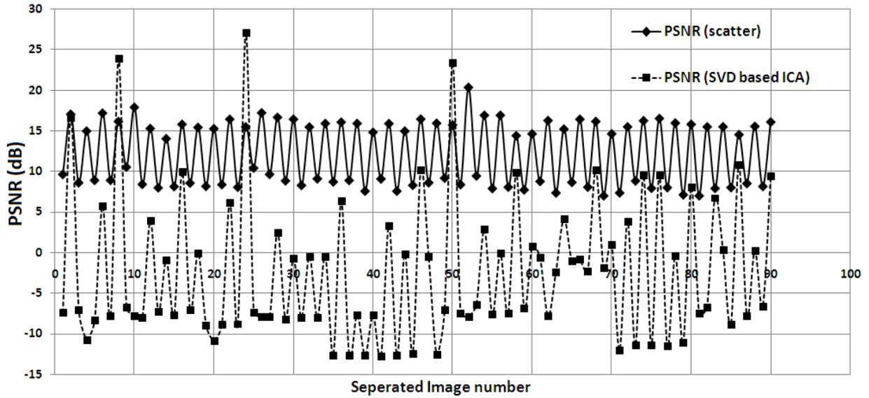
Fig. 6: PSNR for the separated images using scatter-plot based technique and SVD-based ICA techniques.
