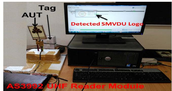
Fig. 16. RFID read range measurement setup.
