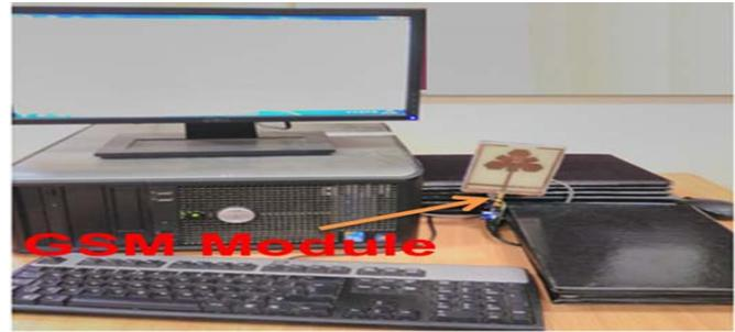
Fig. 18. Antenna with the GSM module.
