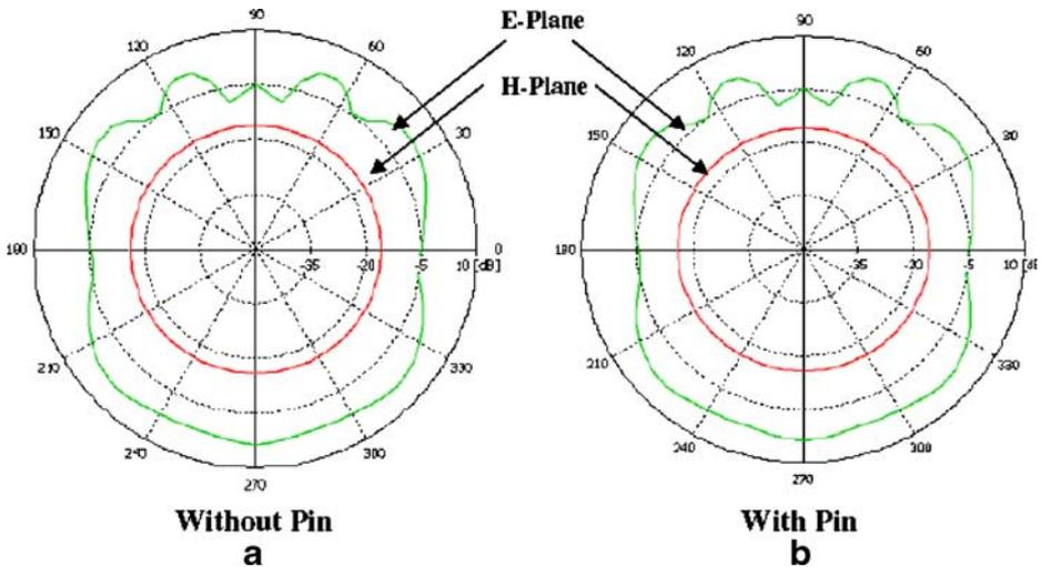
**Fig. 3** E and H plane far-zone radiation pattern for the gain of proposed rectangular microstrip patch antenna at frequency 775 GHz (a) without shorting pin, and (b) with shorting pin.
