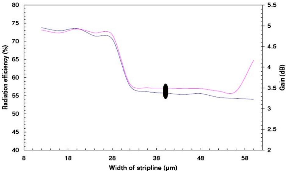
Fig. 5 The effects of variation of width of microstrip-line (feed-line) on the radiation efficiency and gain of the rectangular microstrip patch antenna.
