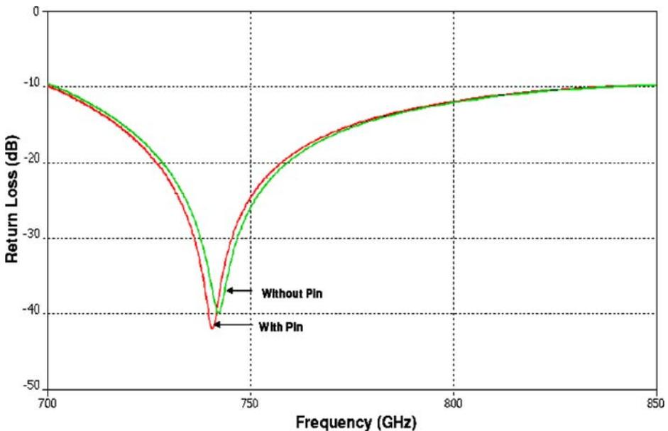
**Fig. 2** Return losses (dB) of the rectangular microstrip patch antenna at THz frequencies for with shorting pin and without shorting pin.
