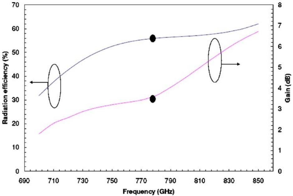
Fig. 4 Variation of the radiation efficiency and gain of the rectangular microstrip patch antenna at THz frequencies.
