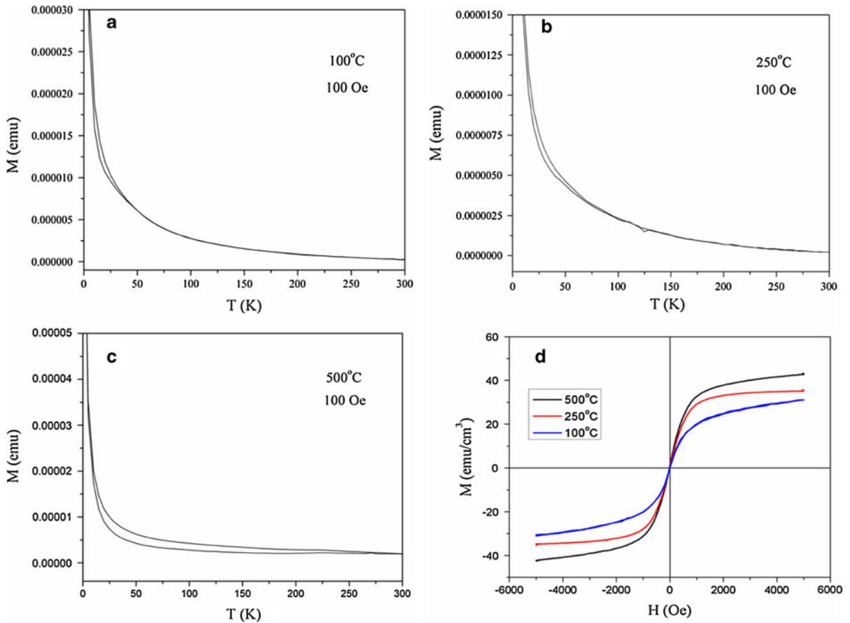
**Fig. 9** M–T plot of the  $\alpha$ -Fe<sub>2</sub>O<sub>3</sub> films annealed at **a** 100 °C, **b** 250 °C, and **c** 500 °C temperatures. **d** M–H plot of these films at room temperature
