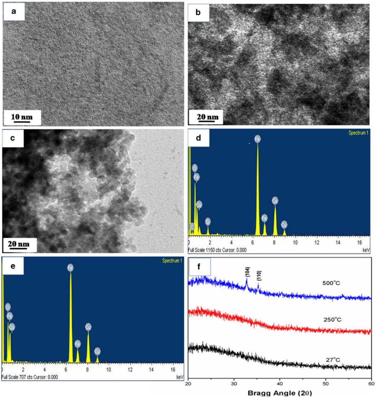
**Fig. 8** a–c TEM images of unheated and annealed films at 250 and 500 °C temperatures. **d** EDX of the unheated film and **e** EDX of the film annealed at 500 °C temperature. **f** the XRD
