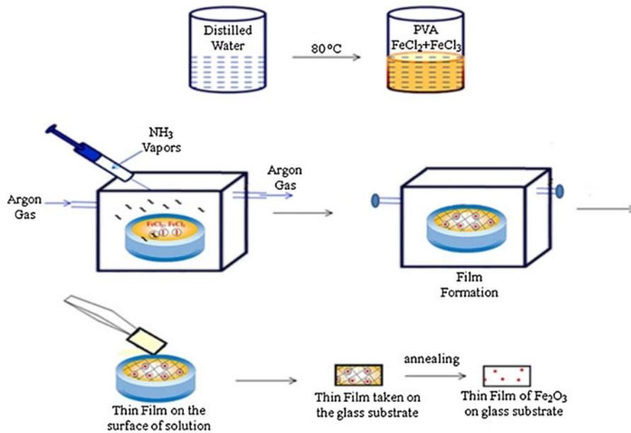
**Fig. 1** Schematic illustration of nanosized hematite ( $\alpha$ -Fe<sub>2</sub>O<sub>3</sub>) film formation on a liquid–vapor interface
