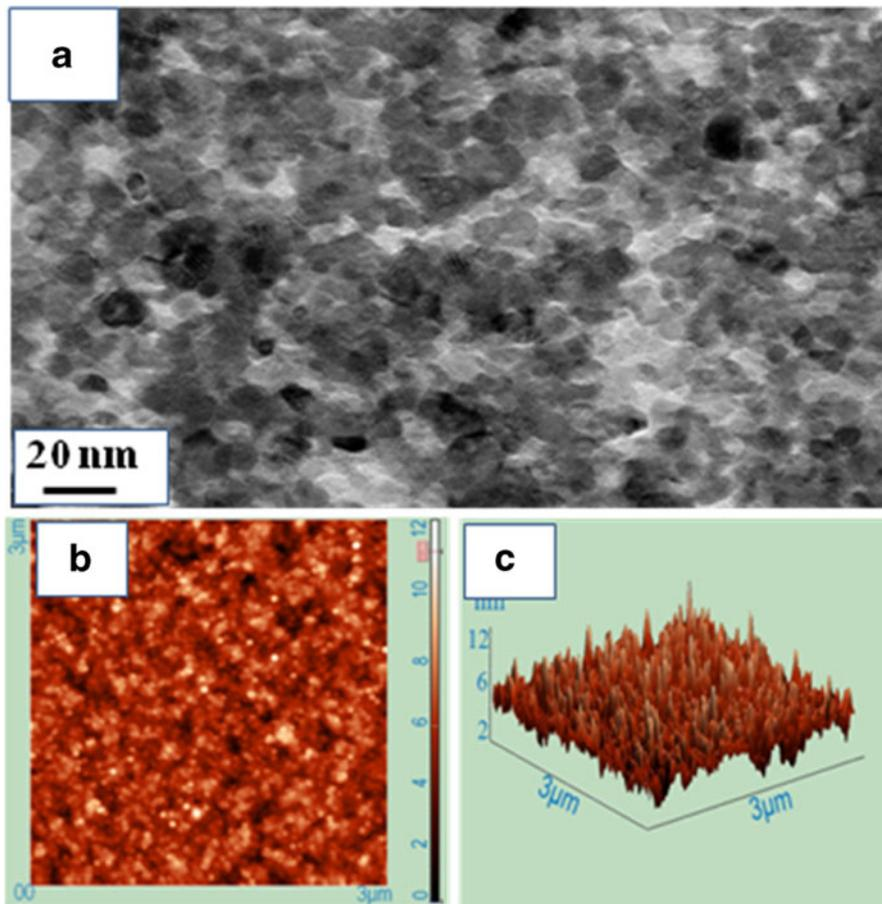
**Fig. 4** **a** TEM image of the film formed for 4 %  $\text{NH}_3$  vapor and 32  $\mu\text{M}$  concentration of PVA, **b** AFM amplitude image, and **c** three-dimensional AFM image of the film
