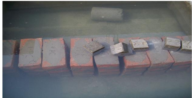
Fig. 8 Curing in laboratory
