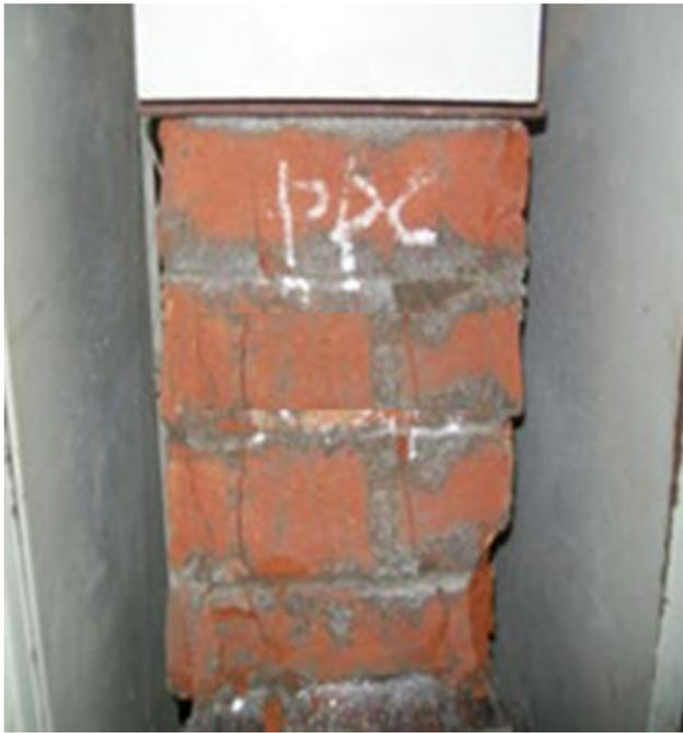
**Fig. 14** Experimental verification of XY shear
