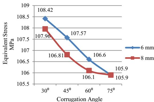
**Fig. 7** Equivalent stress vs corrugation angle for variable web thickness of 150 mm plate length and 35 mm web width
