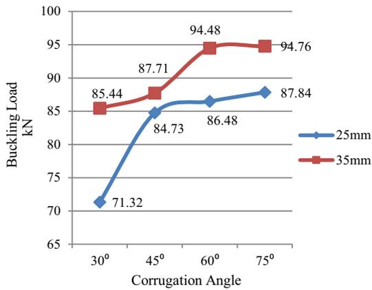
**Fig. 11** Buckling load vs. corrugation angle for variable web width of 150 mm plate length and 6 mm web thickness
