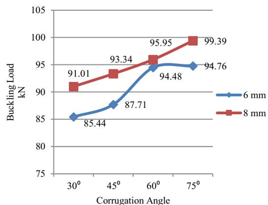
**Fig. 5** Buckling load vs corrugation angle for variable web thickness of 150mm plate length and 35 mm web width
