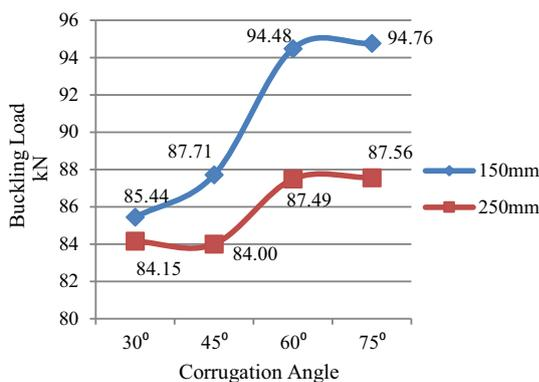
**Fig. 8** Buckling load vs corrugation angle for variable Corrugation plate length of 35 mm web width and 6 mm web thickness
