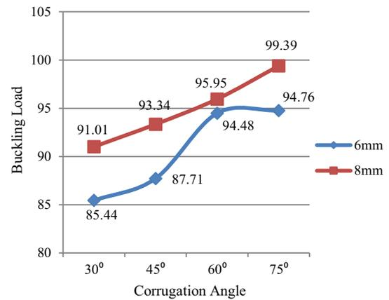
**Fig. 14** Buckling load vs. corrugation angle for variable web thickness of 150 mm plate length and 35 mm web width
