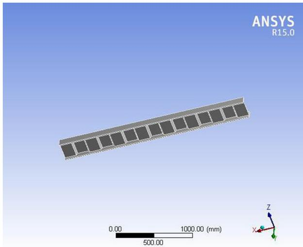
**Fig. 2** Trapezoidal corrugation of the proposed web of the I beam
