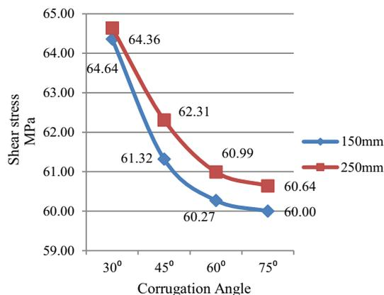
**Fig. 9** Shear stress vs corrugation angle for variable Corrugation plate length of 25 mm web width and 6 mm web thickness
