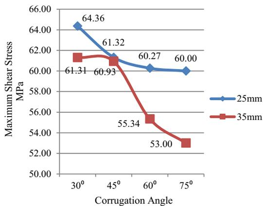
**Fig. 12** Shear stress vs. corrugation angle for variable web width of 150 mm plate length and 6 mm web thickness
