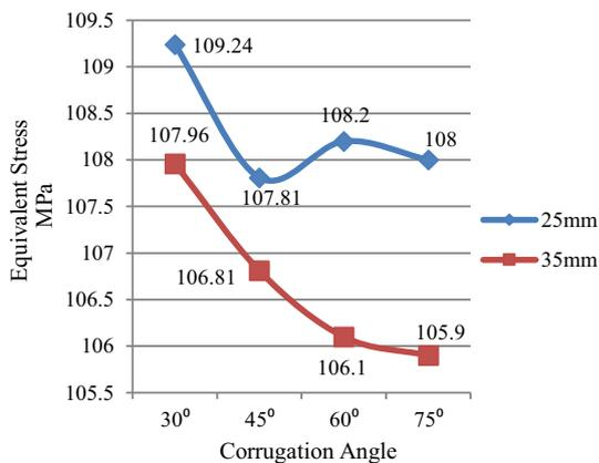
**Fig. 13** Equivalent stress vs. corrugation angle for variable web width 150 mm plate length and 8 mm web thickness
