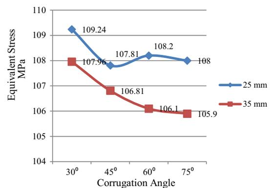
**Fig. 16** Equivalent stress vs. corrugation angle for variable web thickness 150 mm plate length and 8 mm web thickness
