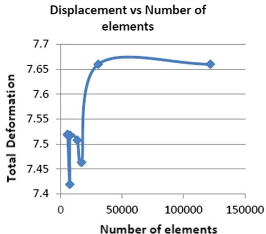
**Fig. 4** Convergence study for Finite element analysis
