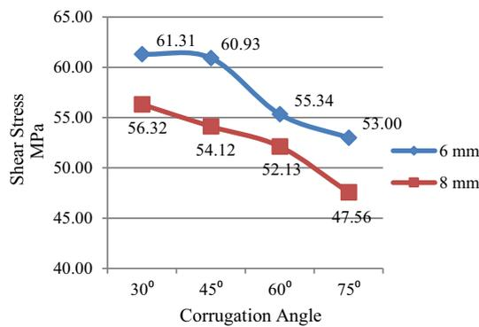
**Fig. 6** Shear stress vs corrugation angle for variable web thickness of 150 mm plate length and 35 mm web width
