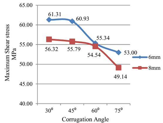
**Fig. 15** Maximum shear stress vs. corrugation angle for variable web thickness of 150 mm plate length and 35 mm web width
