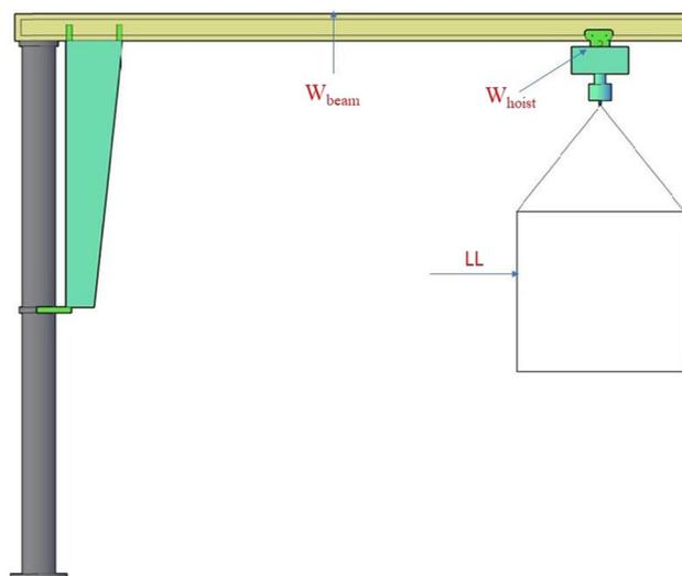
**(a)** Pictorial view of a jib crane with different loading conditions
