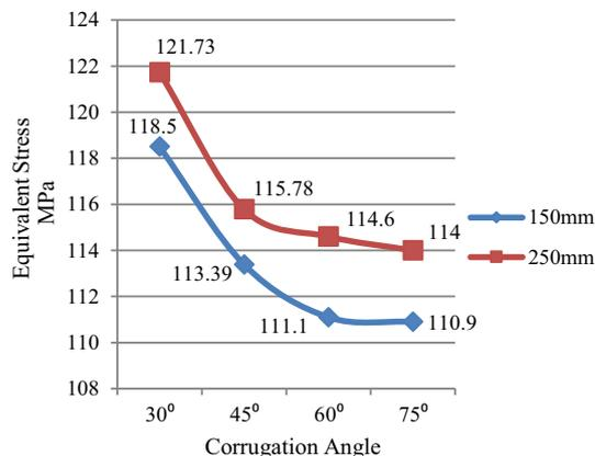
**Fig. 10** Equivalent stress vs corrugation angle for variable Corrugation plate length 25 mm web 150 mm plate length and 35 mm web width and 6 mm web thickness
