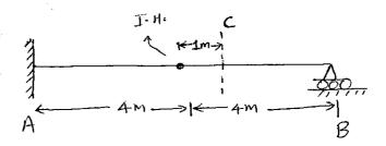
Q4. A triangular load is moving from left to right on the given beam. Find the maximum value of  $R_B$ ,  $R_D$  and bending moment at section C. CO-1, CO-2 [5]
