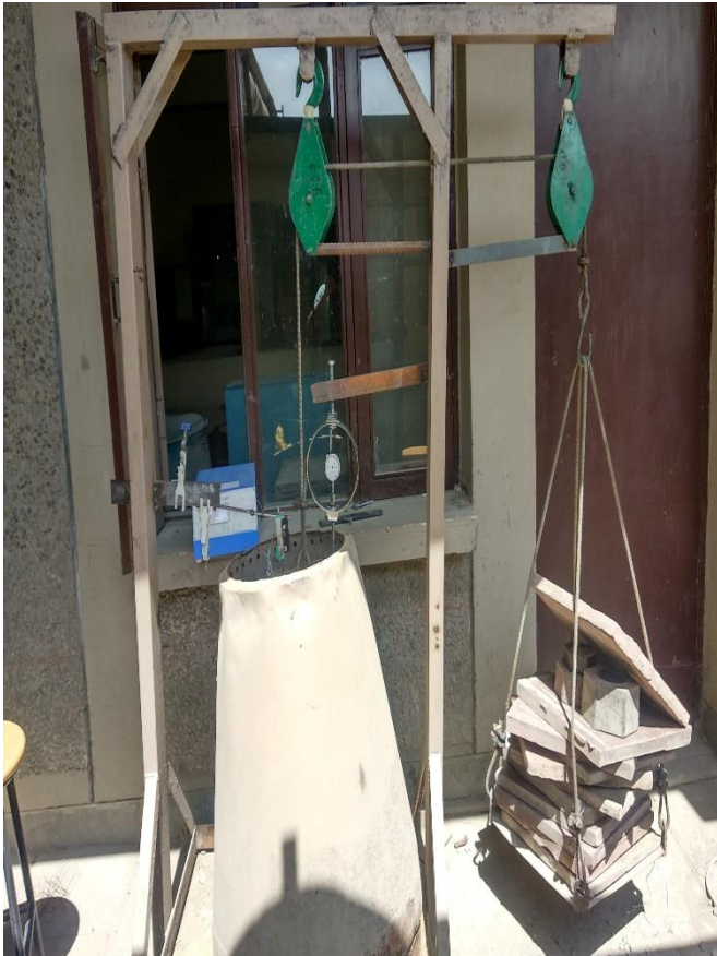
Figure 3.16 - Upliftment of group pile
