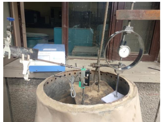
Figure 3.18 - Set up for pile group
