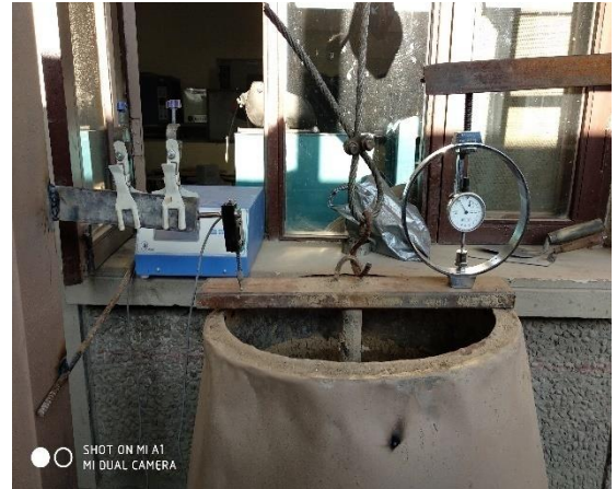
Figure 3.17 - Set up for single pile
