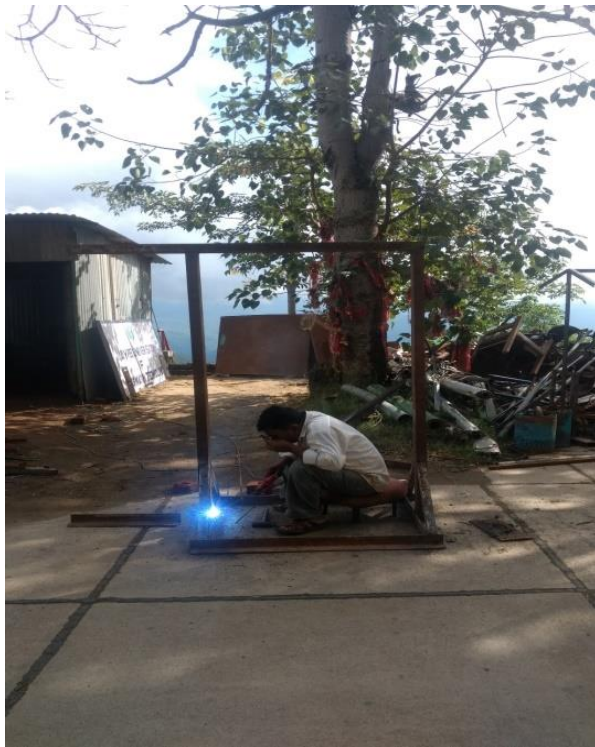
Figure 3.4 - Fabrication of pullout stand
