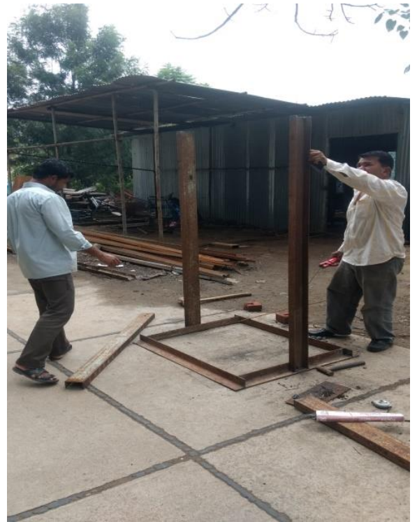
Figure 3.4 - Fabrication of pullout stand
