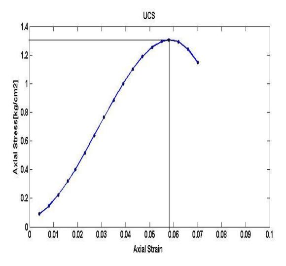
Fig 4. Compressive strength of soil
