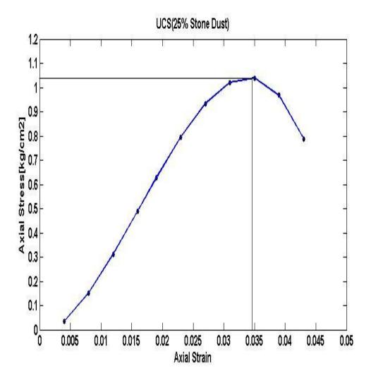
Fig 12. Compressive Strength of soil with 25% stone dust
