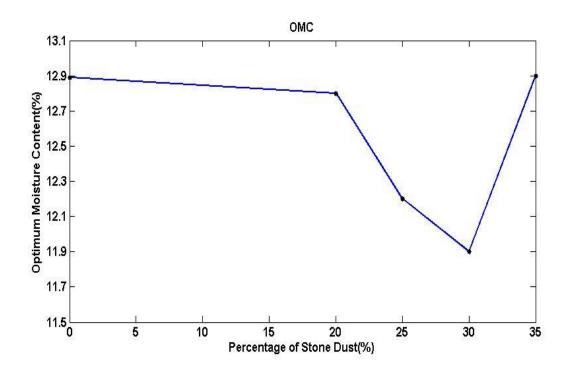
Fig 21. Variation of optimum moisture content with % of stone dust
