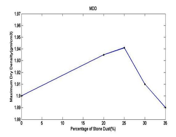
4.1 Effect of Stone Dust on Maximum Dry Density and Optimum Moisture Content
