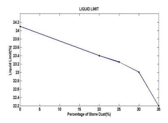
Fig 25. Variation on Liquid Limit with % of stone dust
