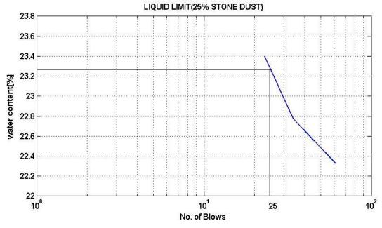
Fig 17. Liquid Limit of soil with 25% stone dust
