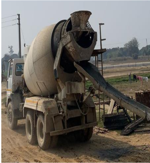
Figure 3.1.8 Tran mixer (7 cum 2 ) and Concreting of side wall, using vibrator
