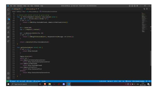
A handler layer has the main functions which the url end point points to and is used call the usecase layer which in return calls the repository layer.
