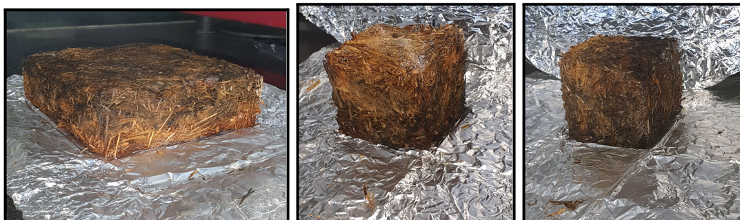
Figure 04.1.a- demoulded and heat killed biocomposite from small wooden mould.
