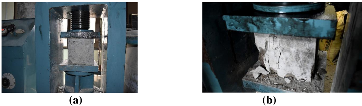
Fig. 4.9 (a) Cubes before application of load, (b) Cubes after application of load
