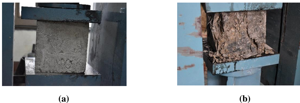
Fig. 4.5 (a) Cubes before application of load, (b) Cubes after application of load
