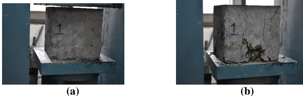
Fig. 4.7 (a) Cubes before application of load, (b) Cubes after application of load
