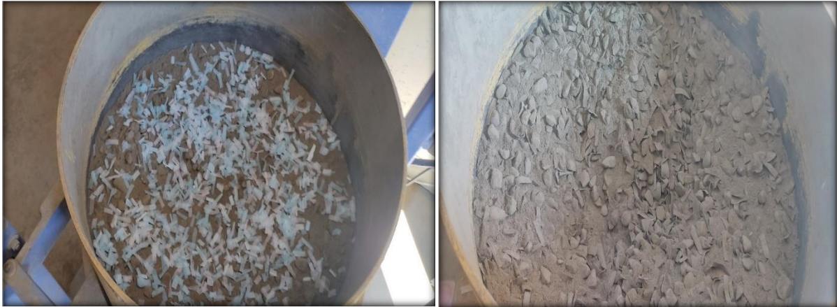
Fig 3.6: Dry mixing with shredded face mask
