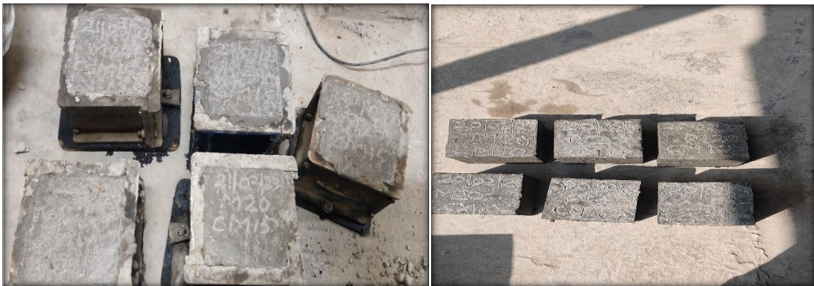
Fig 3.7: Demolding after 24h
