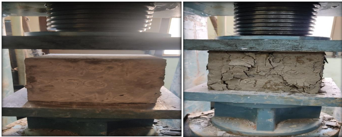
Fig 3.8: Testing of concrete cube
