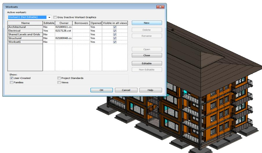
**Figure 8.3** Work sets in Revit
