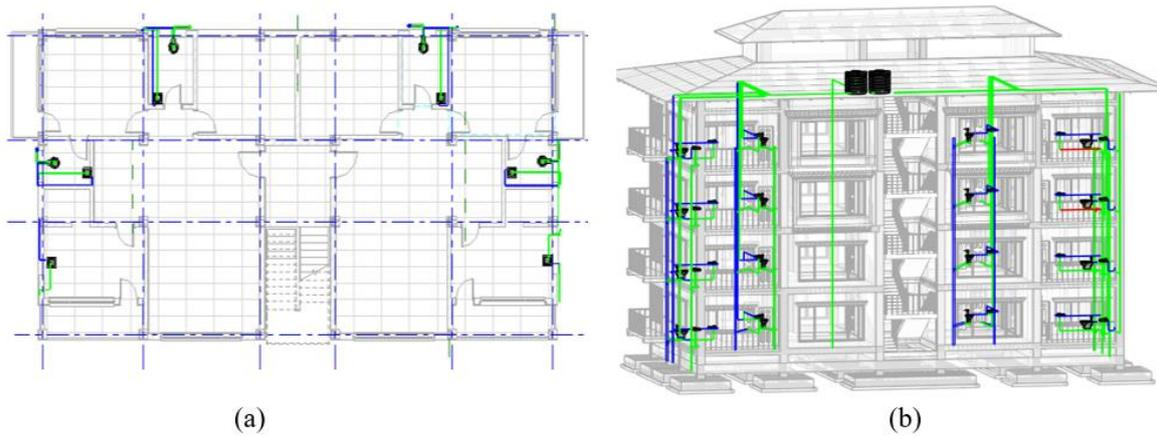
**Figure 4.6** (a, b) Plumbing floor plan and 3D model
