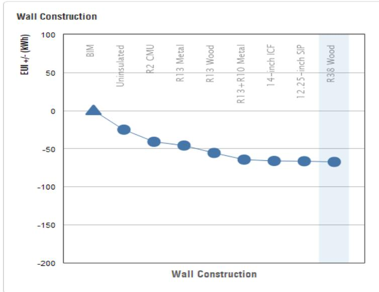
**Figure 9. 13** Wall Construction
