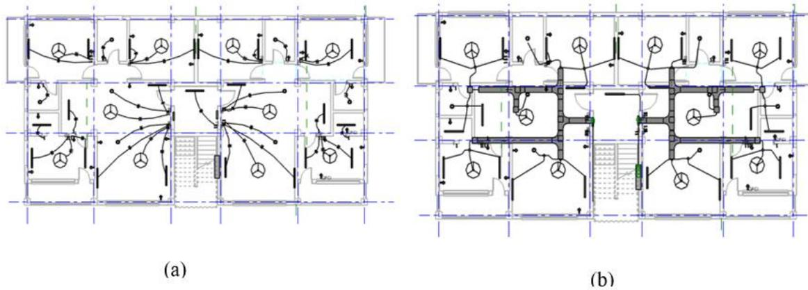
**Figure 4.4** (a, b) Electrical Floor Plan & Ceiling Plan
