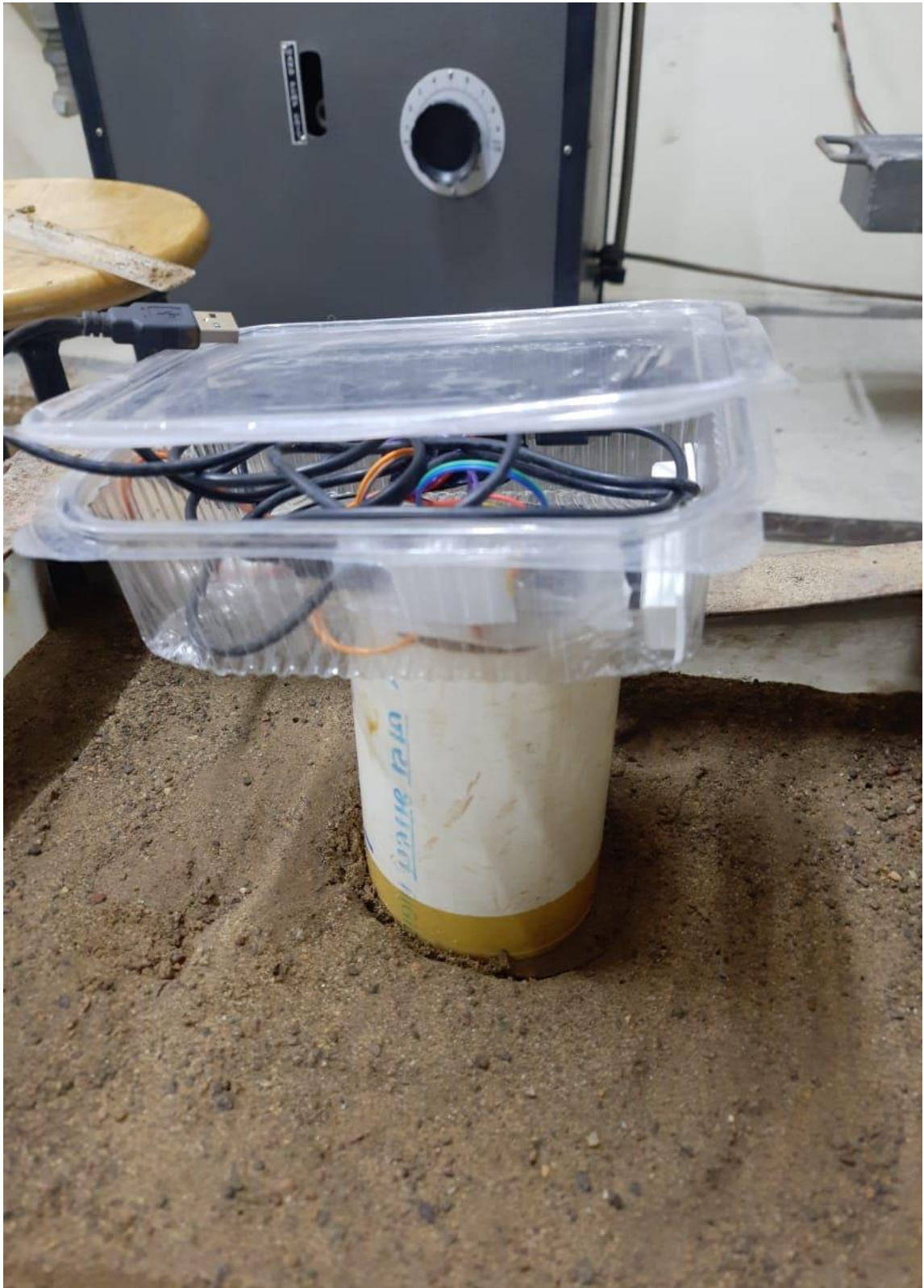
Fig 3.3 Sensors in prototype to record changes.
